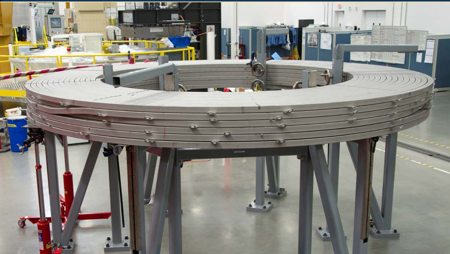
Wound six-layer submodules ready for terminal preparation
