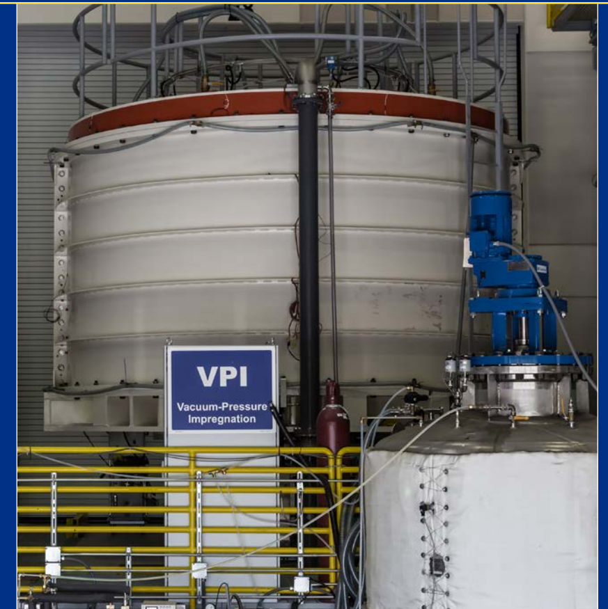
Module mold alongside resin tanks and mixing pump system for injecting 3,500 liters of resin to encapsulate the module
