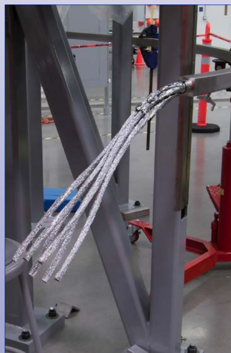
Conductor strands prior to chrome stripping
