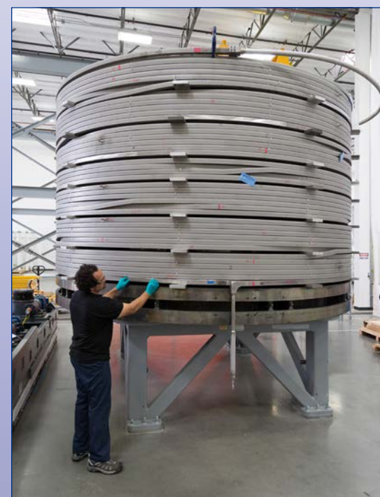
Module with six completed splice joints
