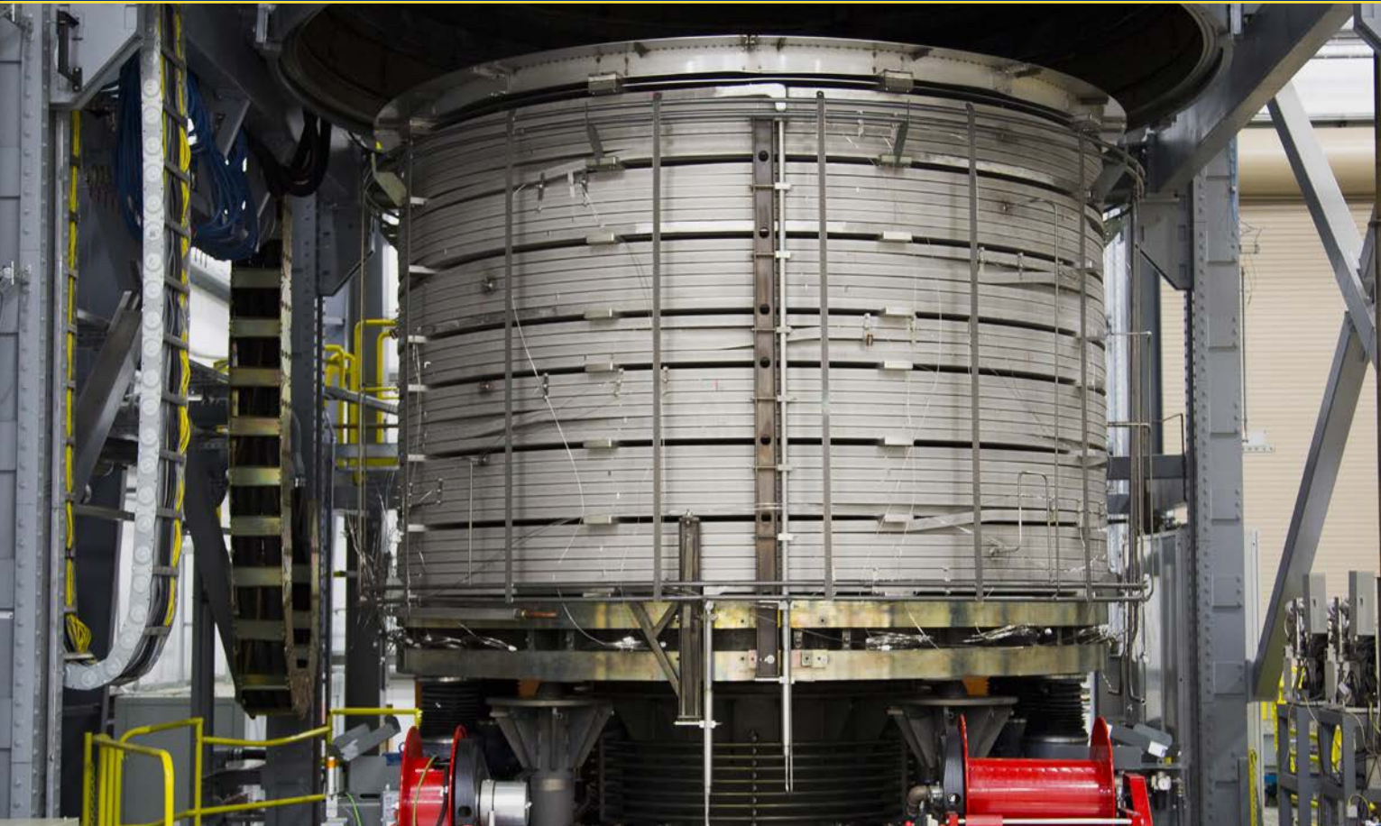
Air transporter placing module in furnace for heat treatment at 650°C (1200°F)
