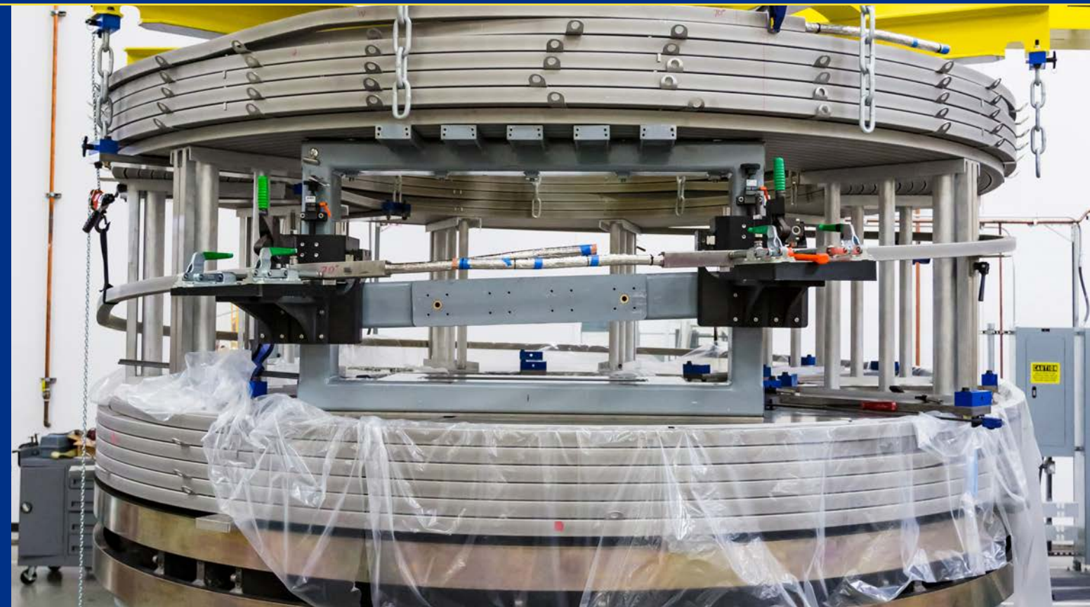
Two hex submodules prepared prior to joining
