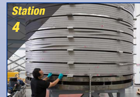
Stack & Join/Helium Penetrations
