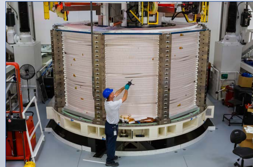
Turn insulation of module nearing completion
