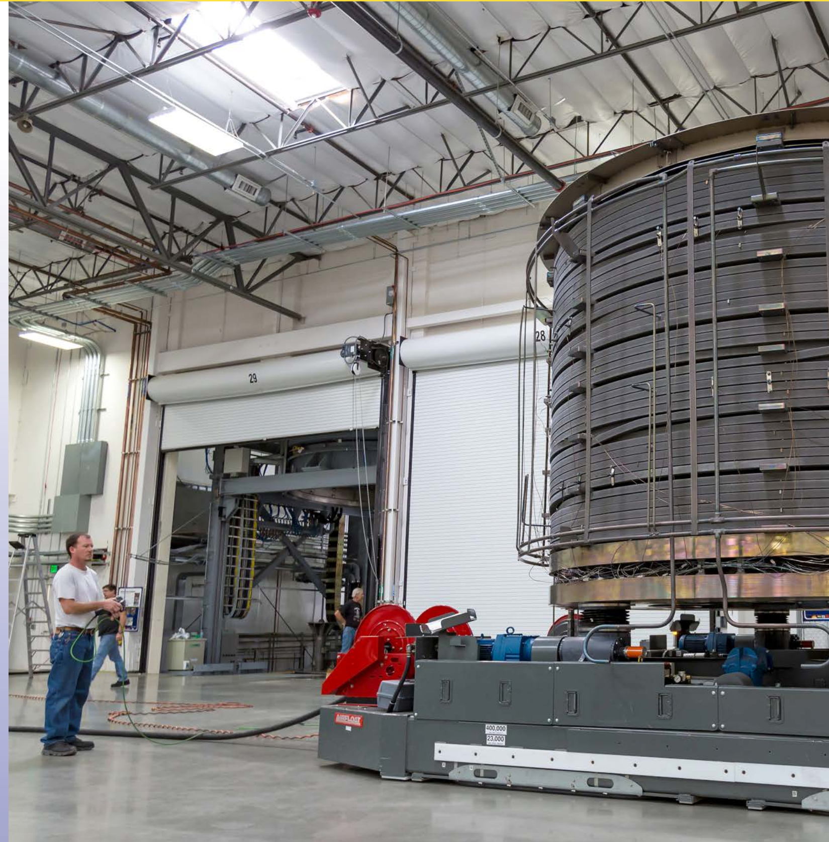
Moving 250,000 lb. (110-tonne) module in facility requires air transporter
