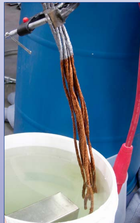
Conductor strands after chrome stripping
