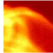
High-speed video image of the MAST plasma obtained at the start of an ELM. The top right hand corner of the photograph has been expanded on the right to highlight the similarity of the ELM filament with a solar eruption.
