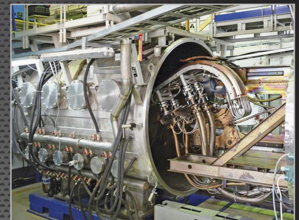
The plasma-facing components of the ITER divertor will sustain the highest head loads of the ITER machine. In St. Petersburg, Russia, an 800 kW electron injector tests prototypes by subjecting them to ITER-like heat loads.
