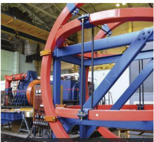
These test stands at the Efremov Institute in Russia are ready to receive key elements of the ITER power supply and superconducting magnet protection system for testing in 2017. *Photo: ITER Russia*
