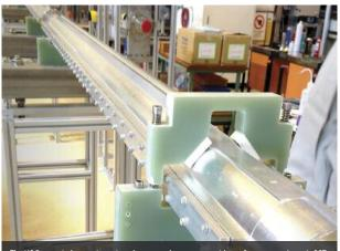
The US Domestic Agency is testing electron cyclotron waveguide performance at Japan's QST, the National Institute for Quantum and Radiological Science and Technology. The electron cyclotron system is one of three external heating systems at ITER. *Photo: US ITER*
