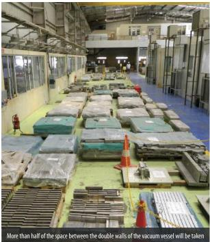
up by in-wall shielding blocks designed to protect ex-vessel components from neutron radiation. Indian contractors are producing over 9,000 elements. *Photo: ITER India*
