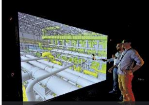
Engineers at ITER use virtual renditions of the machine's systems to verify integration issues, interfaces and assembly sequences.
