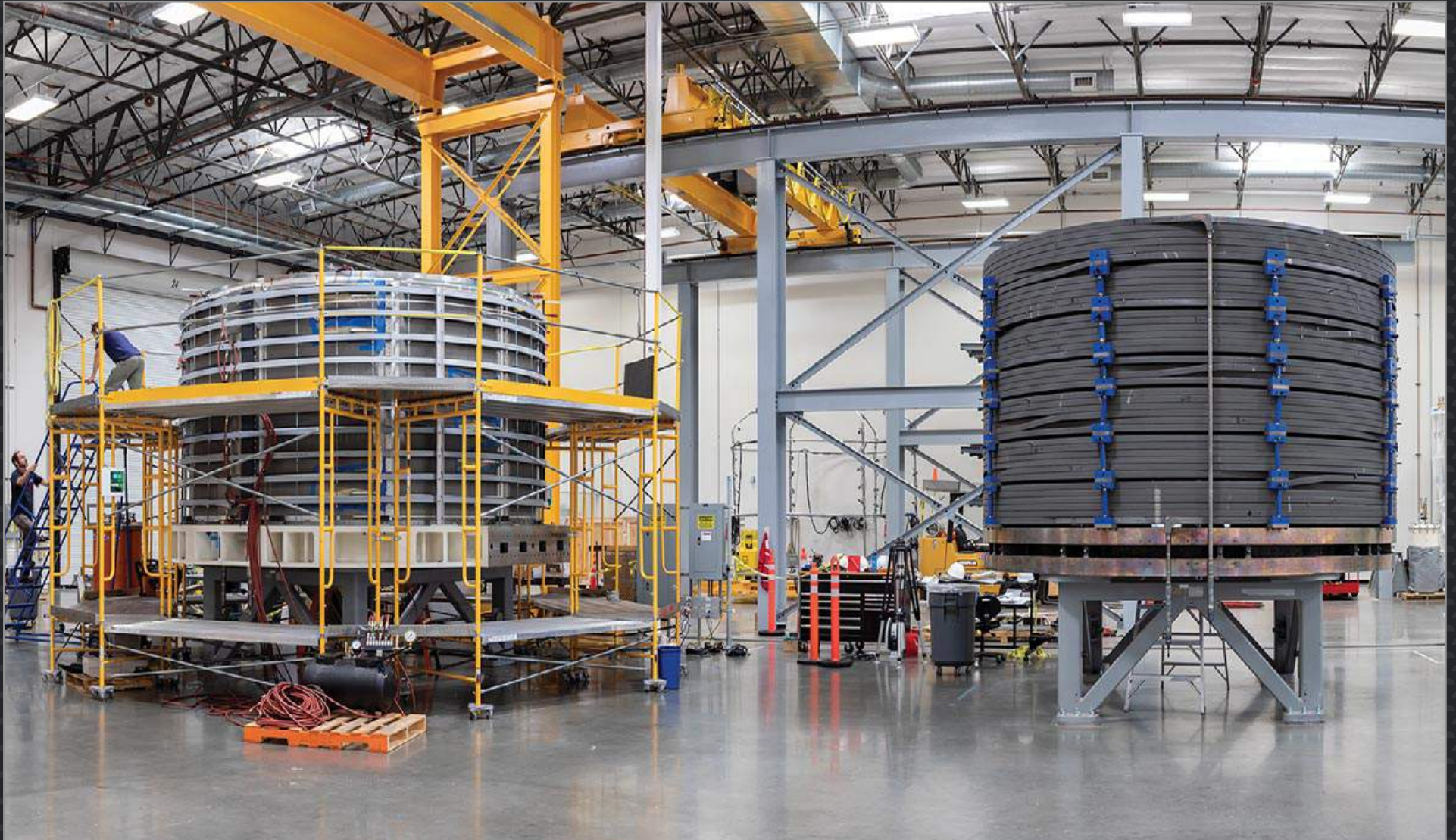
In the General Atomics workshop, one central solenoid module is about to undergo vacuum pressure impregnation (left) and another has been successfully heat treated.
