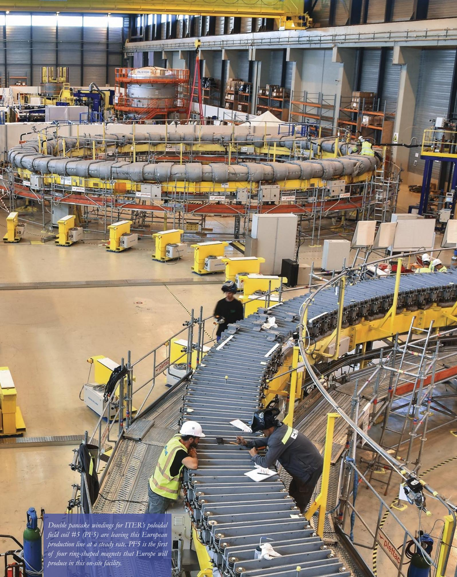
*Double pancake windings for ITER's poloidal field coil #5 (PF5) are leaving this European production line at a steady rate. PF5 is the first of four ring-shaped magnets that Europe will produce in this on-site facility.*
