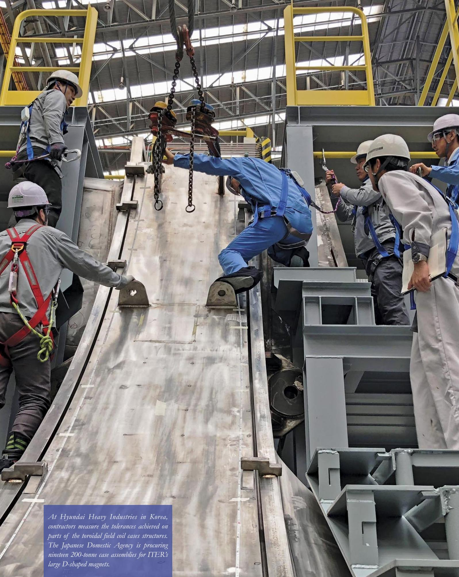
*At Hyundai Heavy Industries in Korea, contractors measure the tolerances achieved on parts of the toroidal field coil cases structures. The Japanese Domestic Agency is procuring nineteen 200-tonne case assemblies for ITER's large D-shaped magnets.*
