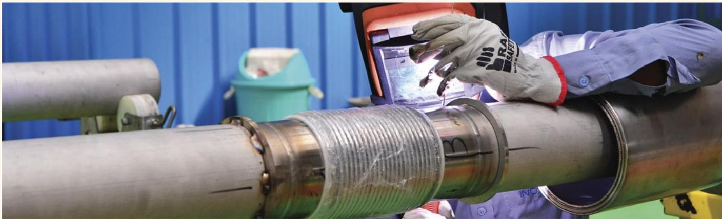
Nearly 5 kilometres of cryolines will transport extremely low-temperature cooling fluids from the ITER cryoplant to client systems in the Tokamak Complex and back. Employees at INOXCVI, based in Vadodra (Gujarat), India, are working to fill approximately half of that order.
