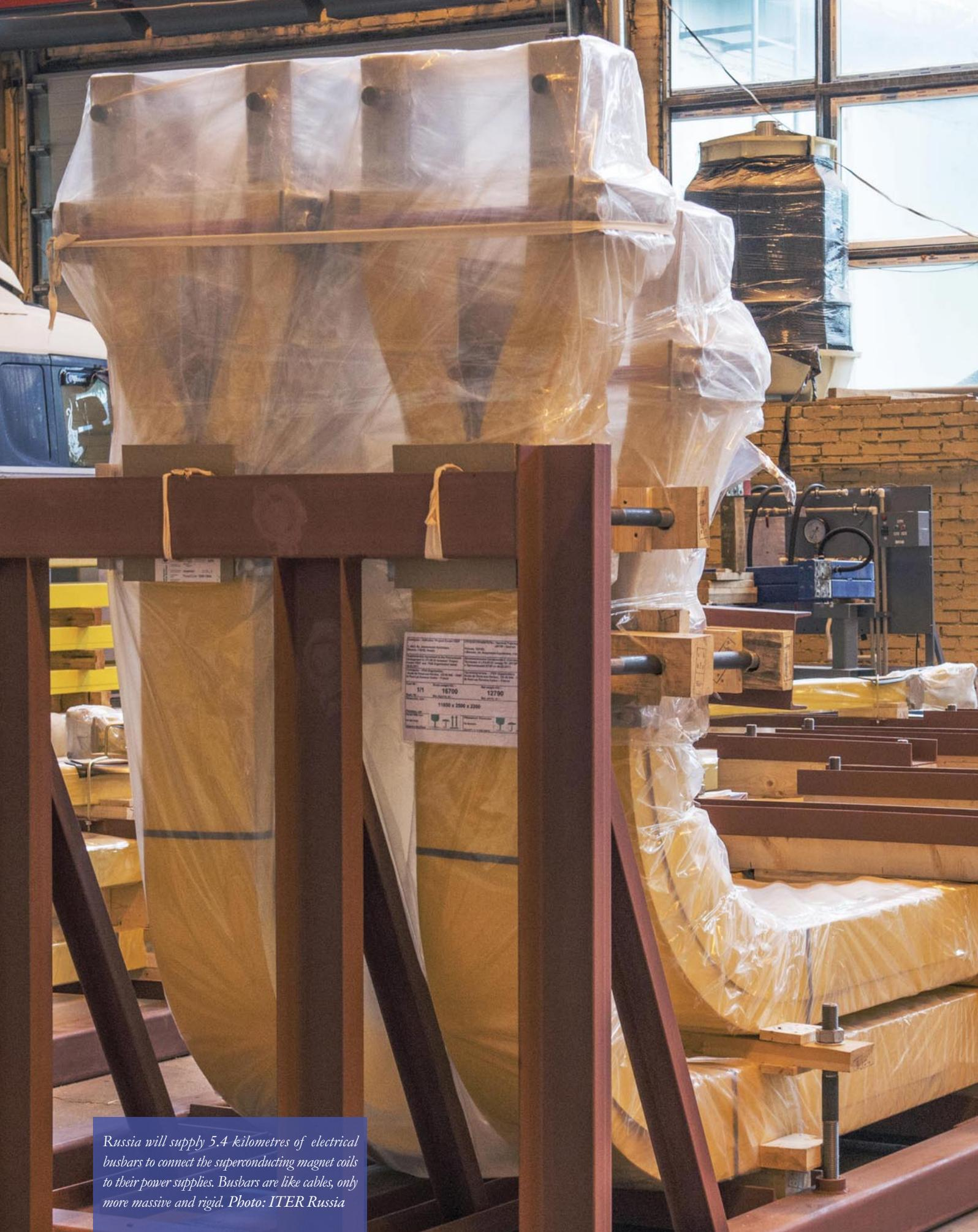
*Russia will supply 5.4 kilometres of electrical busbars to connect the superconducting magnet coils to their power supplies. Busbars are like cables, only more massive and rigid. Photo: ITER Russia*
