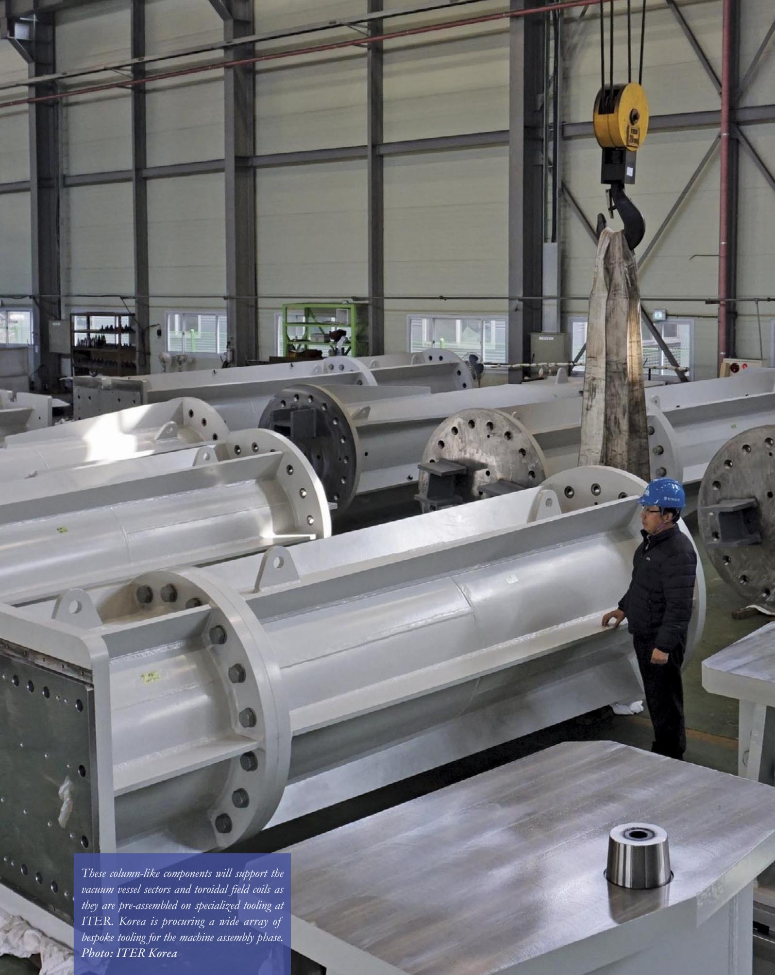
*These column-like components will support the vacuum vessel sectors and toroidal field coils as they are pre-assembled on specialized tooling at ITER. Korea is procuring a wide array of bespoke tooling for the machine assembly phase. Photo: ITER Korea*
