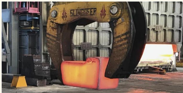
*A secure base and cage will ensure that the 18-metre-tall central solenoid magnet is able to withstand thousands of tonnes of force during operation. One element of the lower support structure is pictured during forging. Photo: US ITER*
