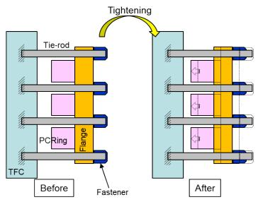
Figure 2-3 TF Pre-Compression Mechanism
