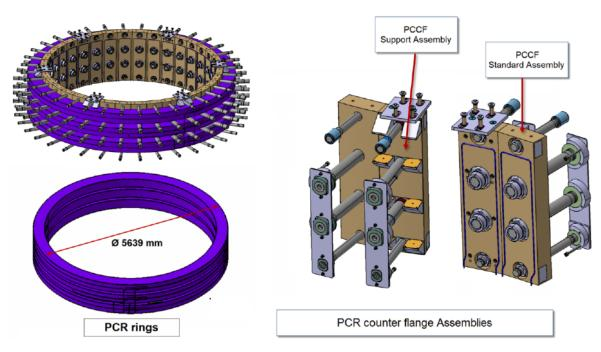
Figure 2-2 Components of TF Pre-Compression System
