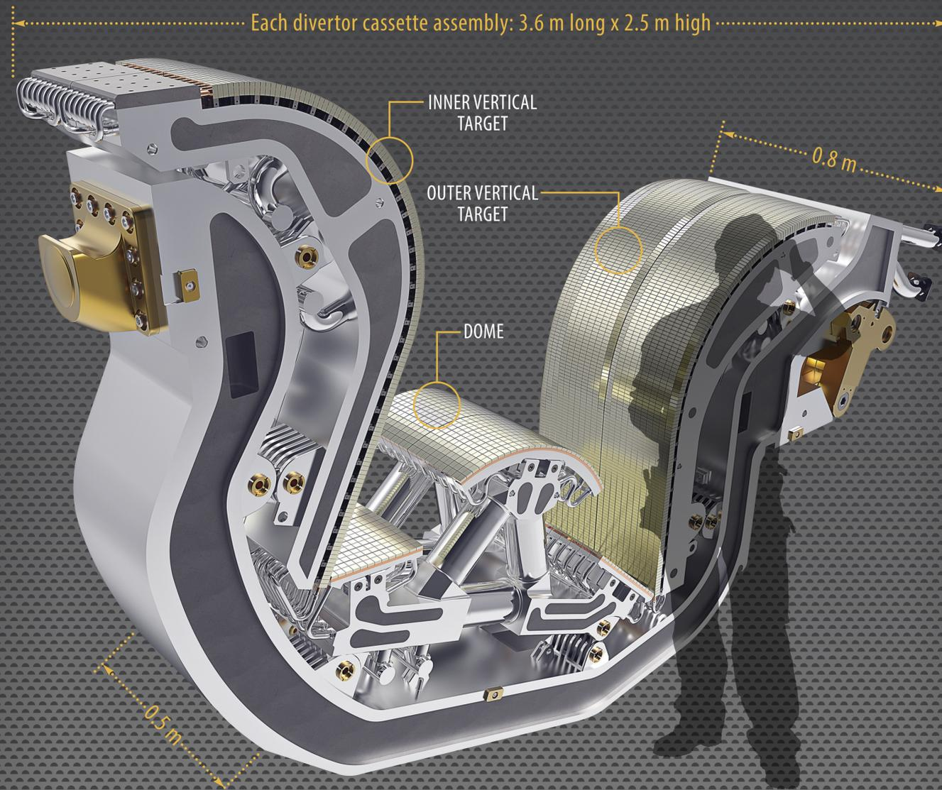
**FIFTY-FOUR 8-TONNE DIVERTOR CASSETTES WILL BE INSTALLED (AND REPLACED) BY REMOTE HANDLING.**
