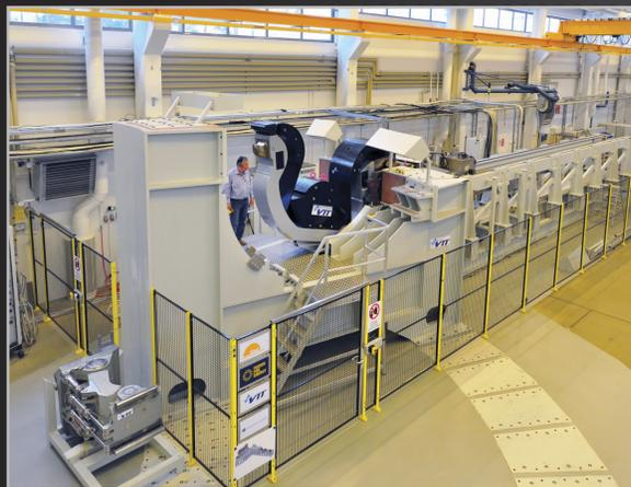
At the DTP2 divertor test platform in Finland, Europe has demonstrated the remote handling operations that will be necessary to install (as well as replace) the eight-tonne divertor cassette assemblies. The demonstrations were performed on a full-size mock-up of the cassette multifunctional mover, designed to transport divertor cassettes along a complex trajectory to the installation arena in the plasma chamber.
