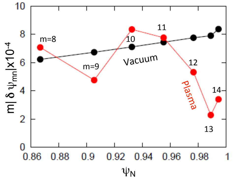
Amplitude of the resonant components v.s. radius in the ELM-suppression  $q_{95}$ -window
