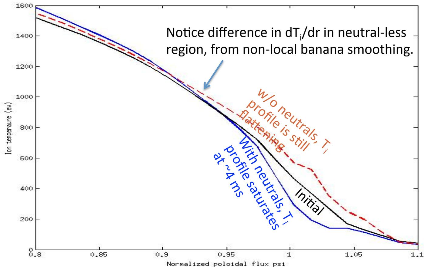
**Cartoon picture of how neutral cooling “bends” down the edge  $T_i$  profile through radial orbital mix**
