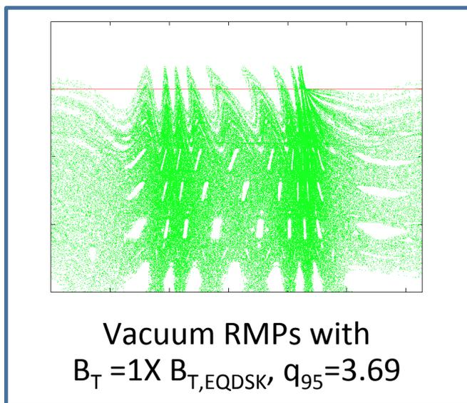
Out-of-window: Field connection between plasma and wall is weak
