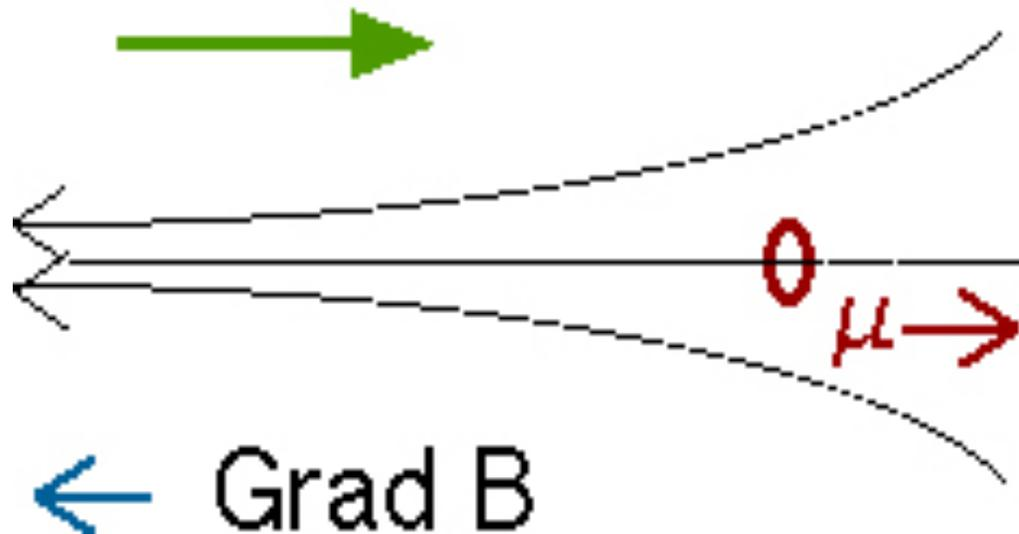
Magnetic mirror force turns particles with small  $v_{\parallel}$  into trapped “banana” orbits. →
