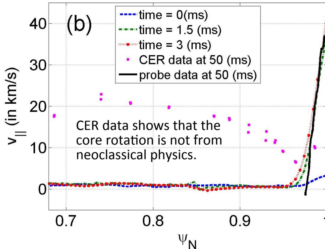
Experimental probe data (black line) in DIII-D agrees with the neoclassical Pfirsch-Schluter flow measurement from XGC1 (green and red dots)
