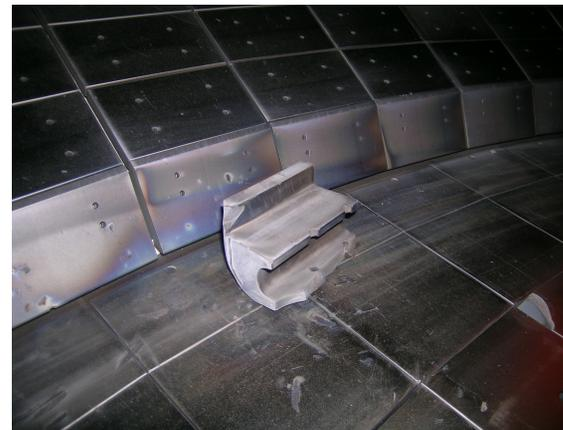
Tile damage due to RE beam on JET
