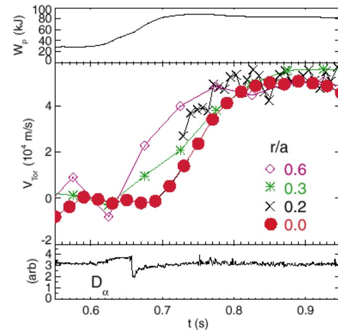
FIG. 1 (color). The plasma stored energy, impurity toroidal rotation velocity at three radii (red dots, green asterisks, and purple diamonds for  $r/a = 0.0, 0.3,$  and  $0.6,$  respectively), magnetic perturbation rotation ( $\times$ ) at the sawtooth inversion radius ( $r/a \sim 0.2$ ), and the edge  $D_\alpha$  brightness for an ICRF heated EDA H-mode discharge.
