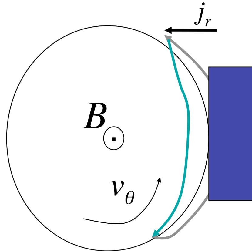
**Poloidal rotation due to the losses of ions interacting with the limiter**
