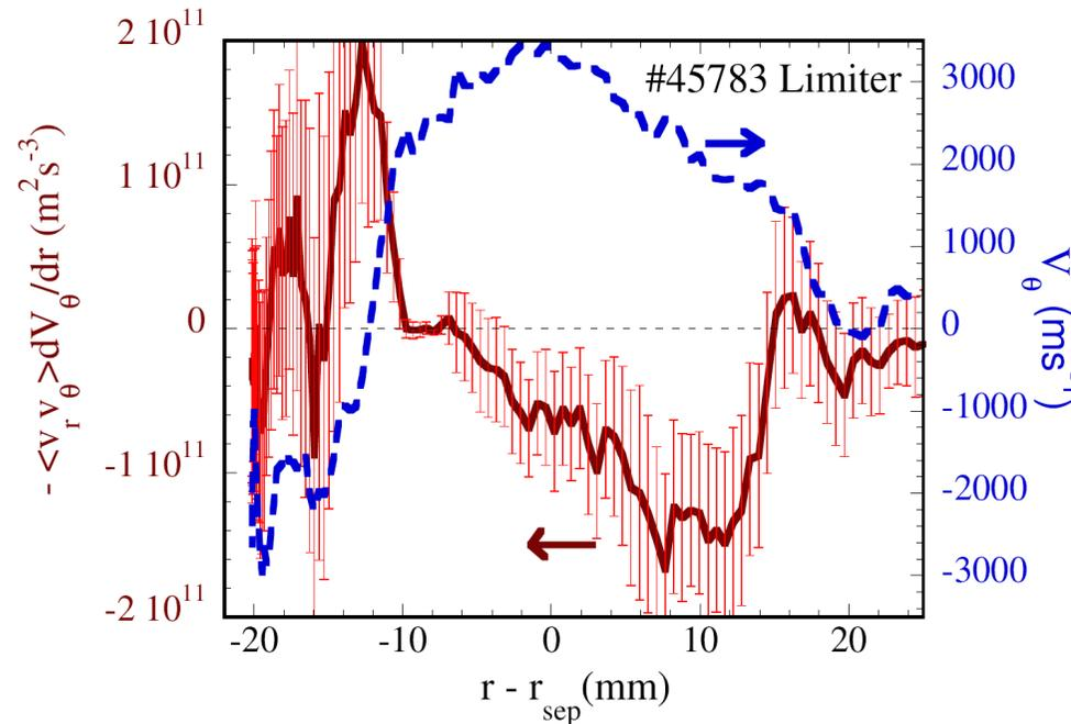
$$P \approx -\langle v_\perp v_r \rangle \frac{\partial V_\perp}{\partial r}$$
