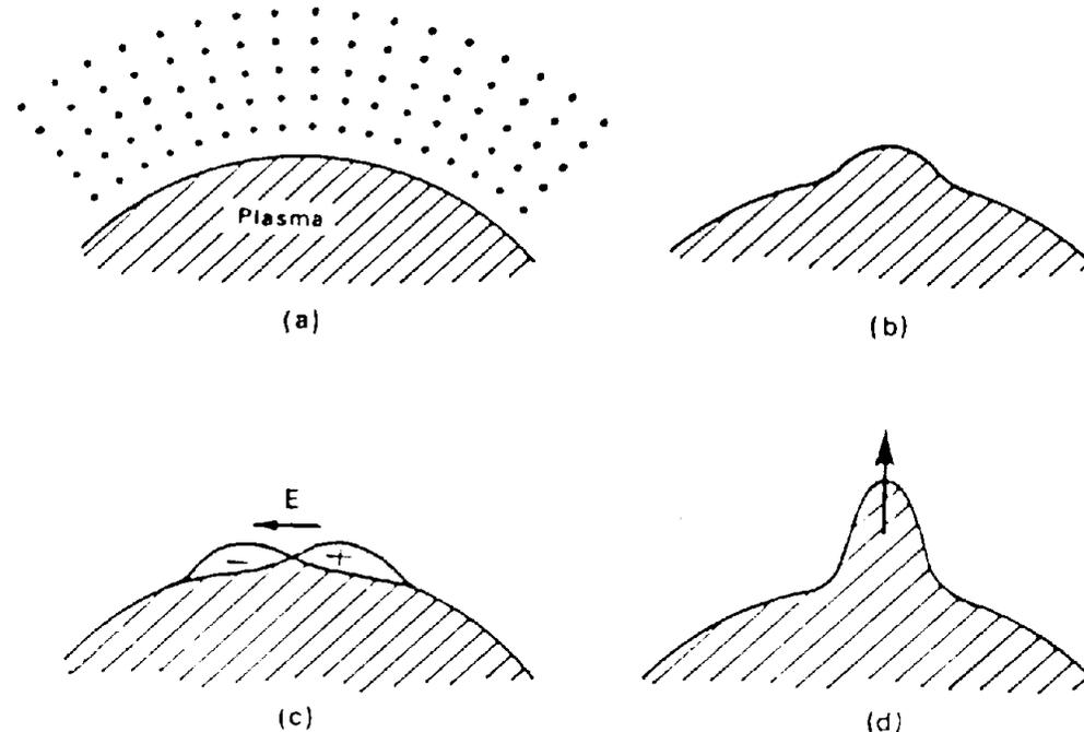
Plasma instability ("interchange instability") can develop in the plasma edge region in the presence of a magnetic field which comes out of the page and decreases with the distance to the plasma boundary (Fig.a).
