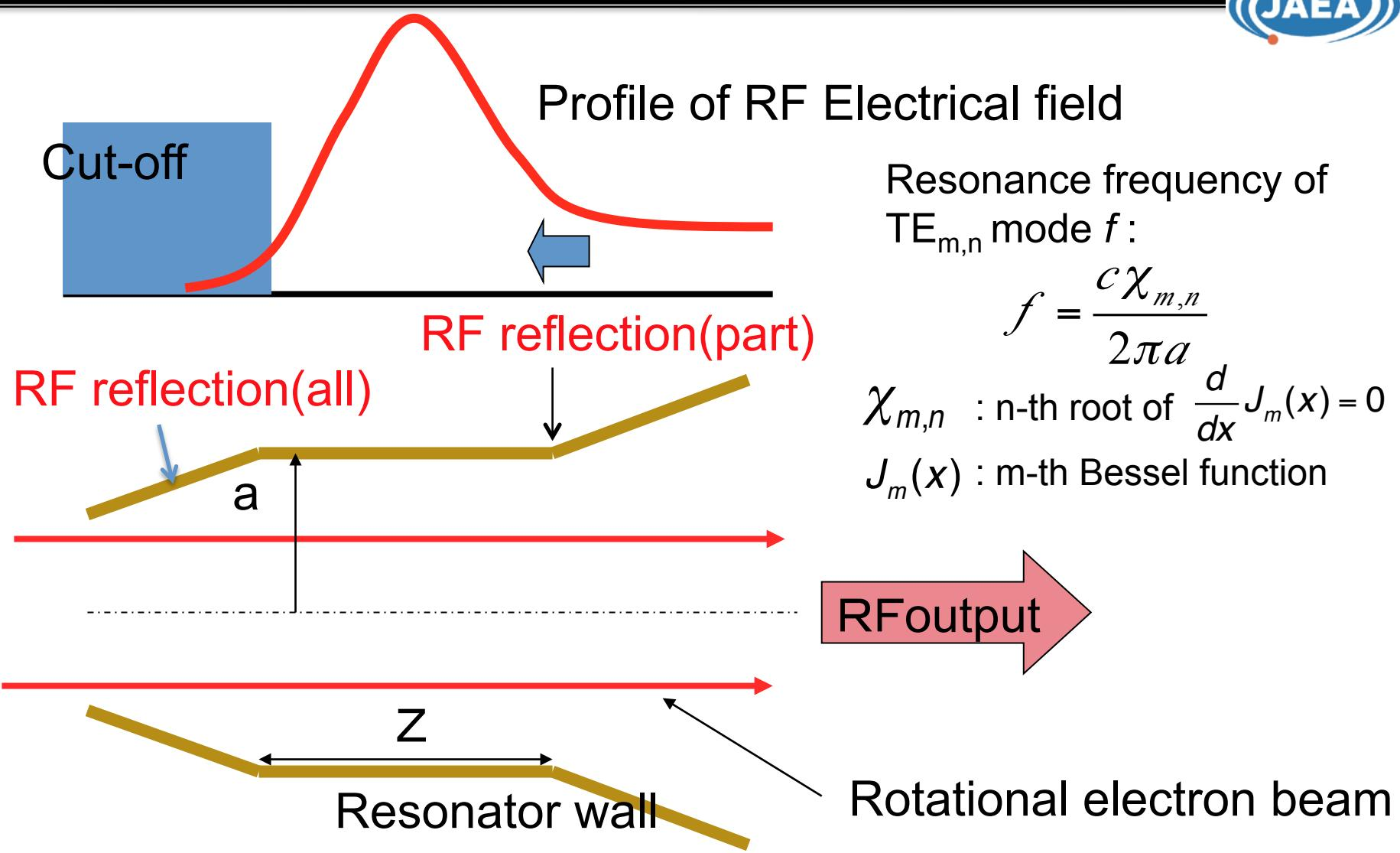
Configuration of gyrotron resonator
