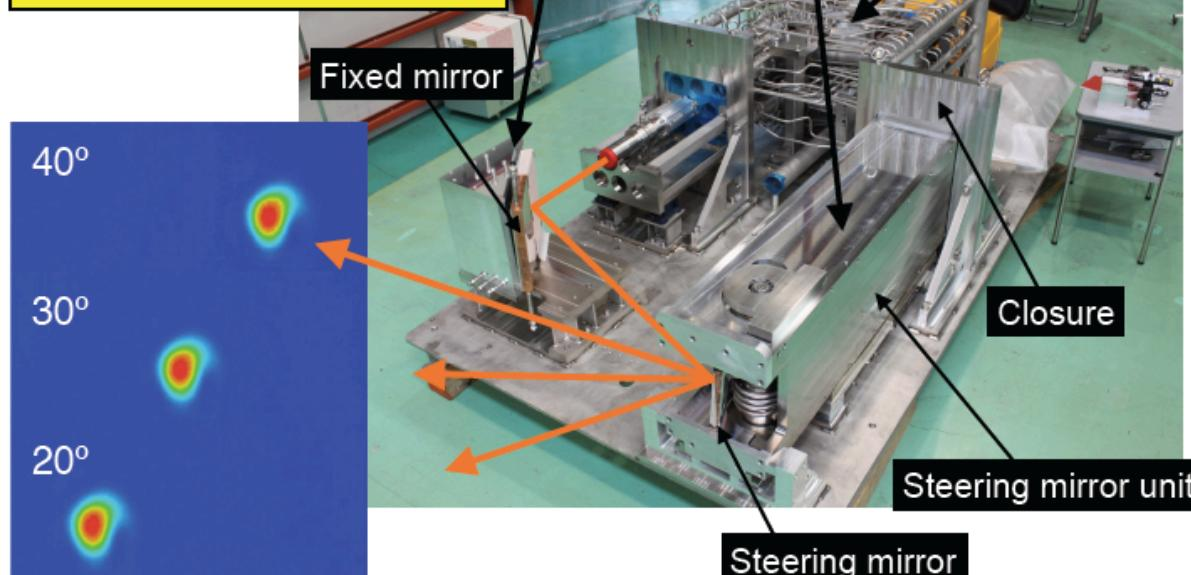
Beam profile at 1.5m from steering mirror (High power test)
