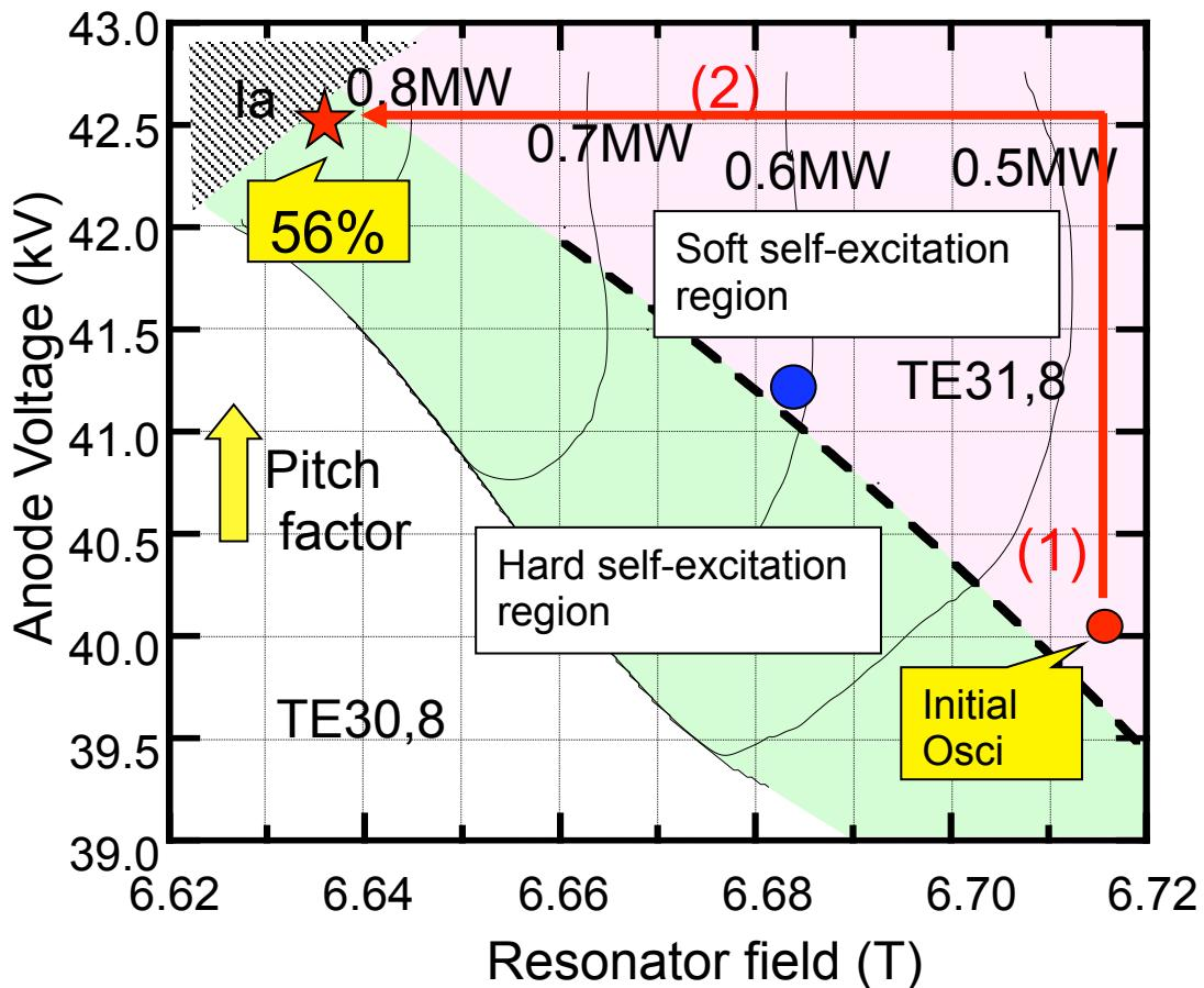
It is proved accessibility to maximum theoretical efficiency by active control.
