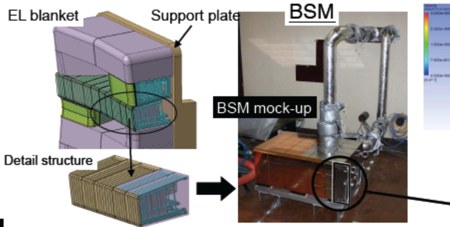
BSM mock-up was fabricated based on the detail design.
