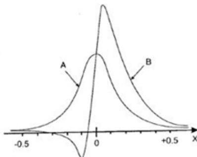
Figure 1. Cyclotron resonance absorption of a non-relativistic (A) and a relativistic (B) electron. The kinetic electron energy in the latter case is 76 eV. The interaction time is close to 1600 wave periods.
