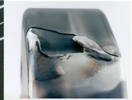
Main Poloidal limiters: VPS-W coated graphite (1998-1999)
