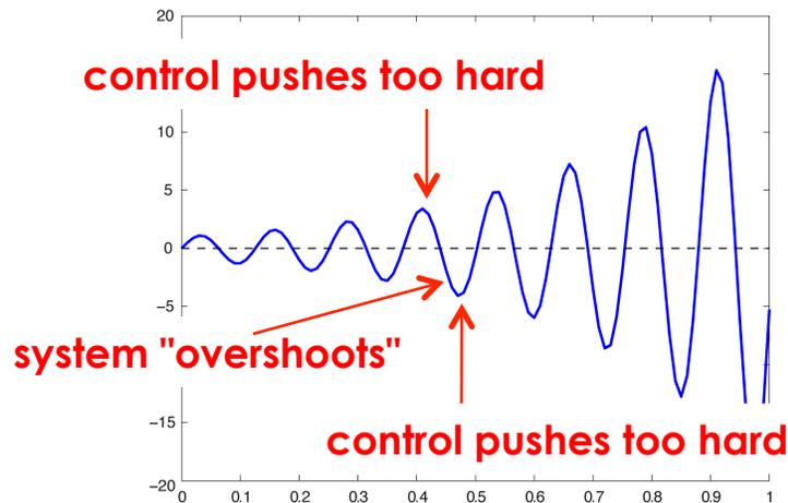
... and closed-loop transfer function has pair of poles in RHP
