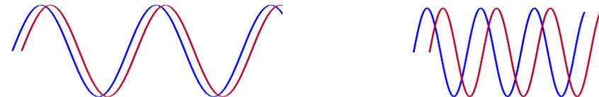
low frequency = small delay, high frequency = large delay
