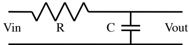
$$\Rightarrow \frac{V_{out}(s)}{V_{in}(s)} = \frac{1}{RCs + 1}$$
