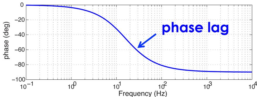
$$\frac{V_{out}(s)}{V_{in}(s)} = \frac{RCs}{RCs + 1}$$
