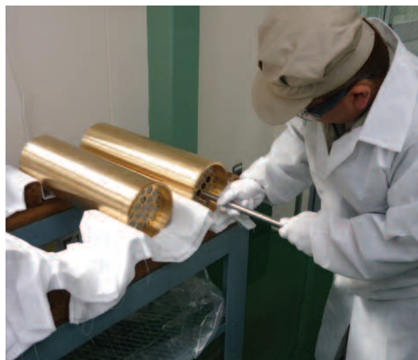
In Japan, workers prepare 40- to 100-kg "billets" of niobium-tin alloy that will be transformed into millimetre-thin superconducting strands for ITER's toroidal field or central solenoid coils. Photo: ITER Japan
