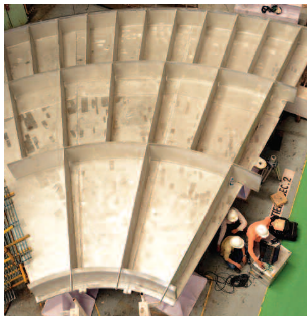
In India, manufacturing activities on the cryostat base progress well in 2014. (Pictured: one of the six 60° base segments, tier 2.) Photo: ITER India
