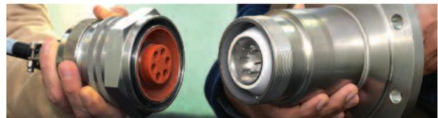
*Magnet instrumentation feedthroughs must operate in an environment characterized by high voltage, high vacuum, high magnetic field and radiation. The first prototypes of these challenging components were delivered for inspection in 2015.*
