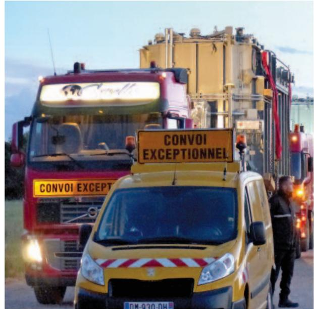
*The ITER Itinerary hosts its first Highly Exceptional Loads in 2015: electrical transformers (pictured) and cooling water tanks procured by the US; water detritiation tanks procured by Europe; and the first cryostat components from India.*
