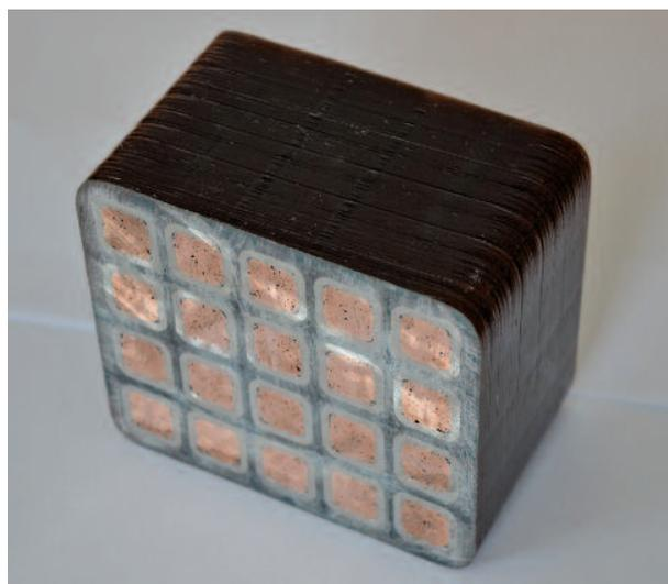
*The first pancakes for ITER's correction coils have been wound in China from niobium-titanium (NbTi) conductor (sample, pictured). The bottom correction coils will be among the first components to be installed during assembly.
