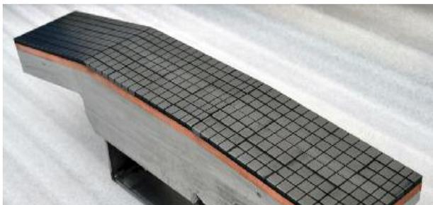
As part of the semi-prototype qualification program in China for enhanced heat flux first wall blanket panels, pairs of beryllium-tiled "fingers" (pictured) have undergone testing at a dedicated facility in Russia. Photo: ITER China
