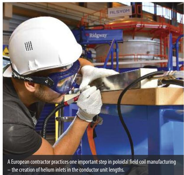
A European contractor practices one important step in poloidal field coil manufacturing – the creation of helium inlets in the conductor unit lengths.
