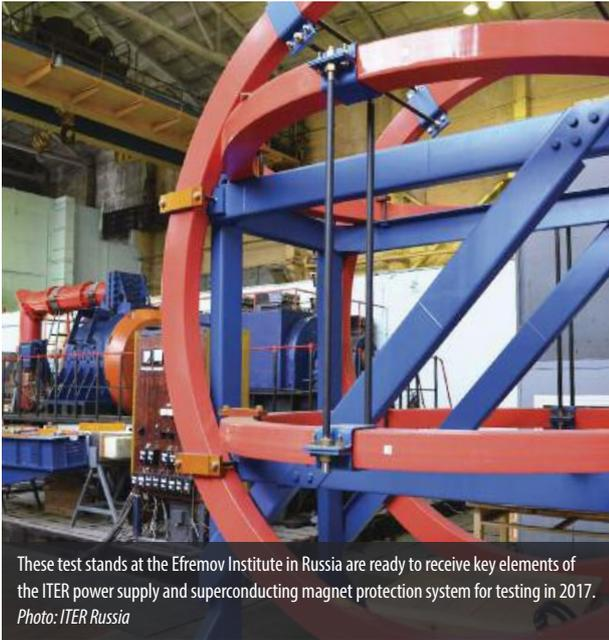
These test stands at the Efremov Institute in Russia are ready to receive key elements of the ITER power supply and superconducting magnet protection system for testing in 2017.
