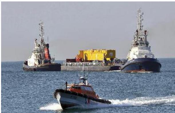
ITER's largest components arrive at the Mediterranean port of Fos-sur-Mer and are transported by barge to the starting point of the ITER Itinerary. From there, they have 104 kilometres to travel to the site. Photo: © ITER Organization - Emmanuel Bonici
