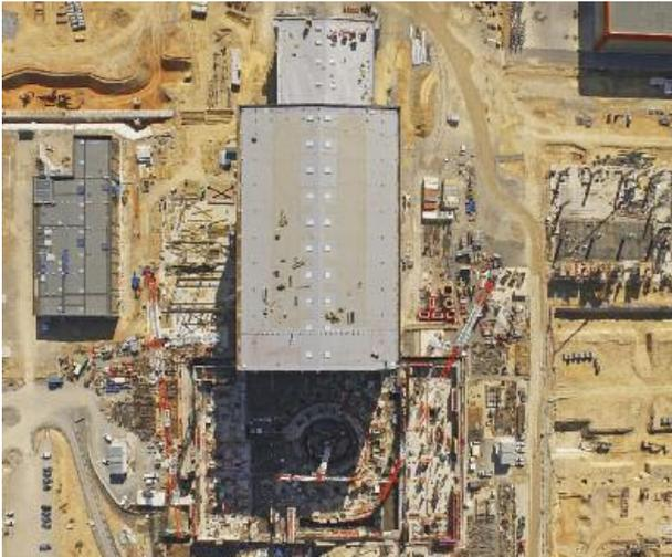
The 17-metre excavation in the platform, the seismic foundations, and the lowest level of the Tokamak Complex are no longer visible as contractors move forward on the Tritium, Tokamak and Diagnostics buildings.
