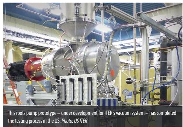
This roots pump prototype – under development for ITER’s vacuum system – has completed the testing process in the US. Photo: US ITER
