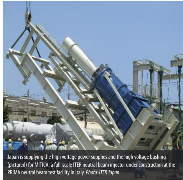
Japan is supplying the high voltage power supplies and the high voltage bushing (pictured) for MITICA, a full-scale ITER neutral beam injector under construction at the PRIMA neutral beam test facility in Italy. Photo: ITER Japan
