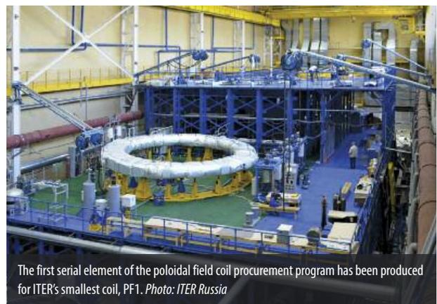
The first serial element of the poloidal field coil procurement program has been produced for ITER's smallest coil, PF1. Photo: ITER Russia
