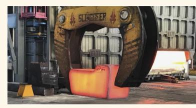
A secure base and cage will ensure that the 18-metre-tall central solenoid magnet is able to withstand thousands of tonnes of force during operation. One element of the lower support structure is pictured during forging. Photo: US ITER
