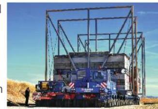
352 wheels, 46 metres long, 9 metres wide, 11 metres high... and 800 metric tons of concrete blocks. ©ITER Organization
