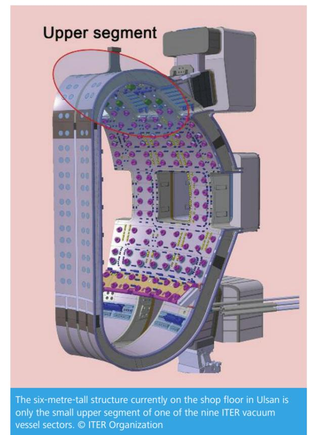
The six-metre-tall structure currently on the shop floor in Ulsan is only the small upper segment of one of the nine ITER vacuum vessel sectors. © ITER Organization
