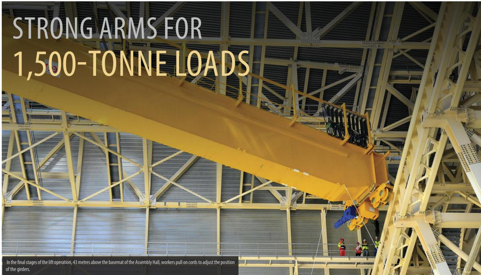
In the final stages of the lift operation, 43 metres above the basement of the Assembly Hall, workers pull on cords to adjust the position of the girders.
