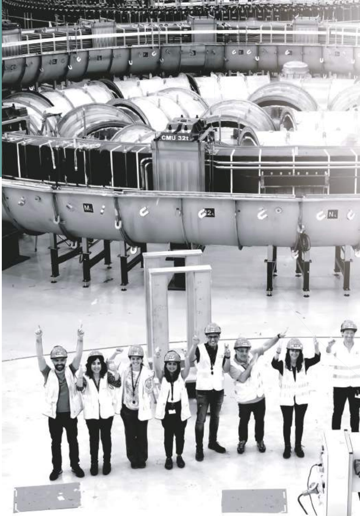
24-metre-diameter poloidal field coil #4 is cold tested successfully mid-year. The European Domestic Agency has one more coil to produce in this facility on site.
