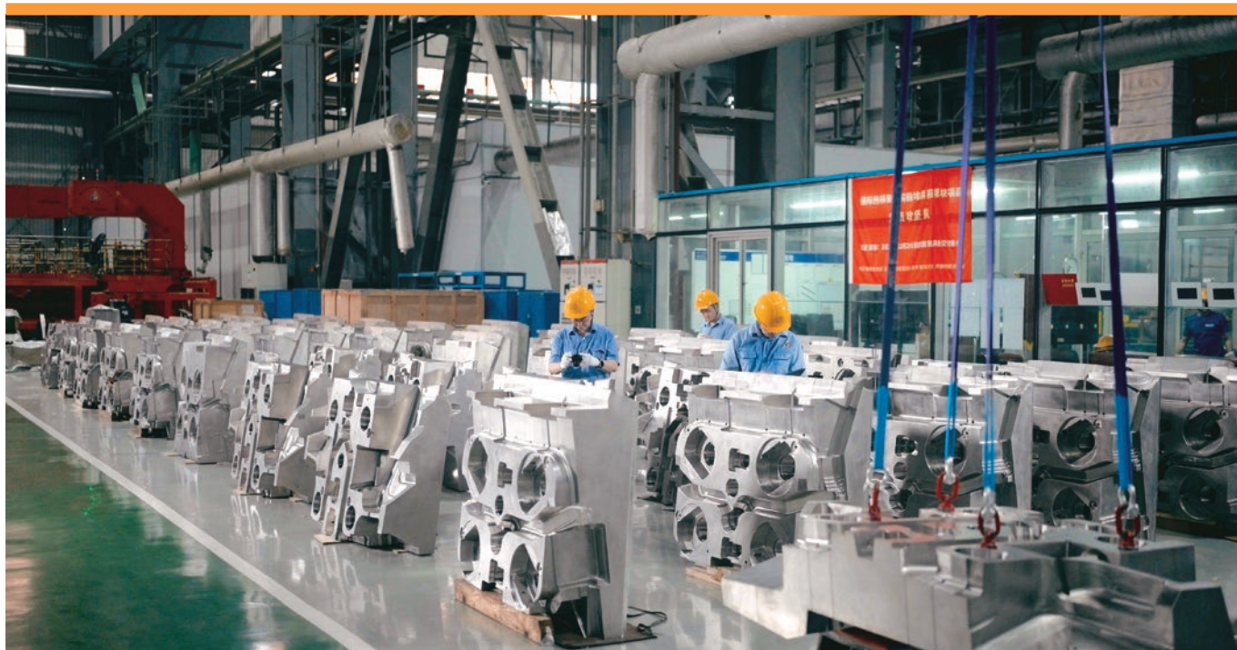
▲ Shield block modules manufactured in China for the ITER blanket.
