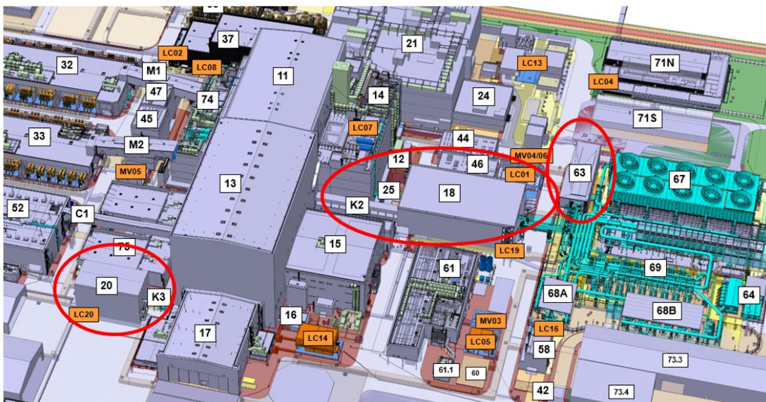
Fig. 7.1.11.2. New buildings and bridges in ITER 2024 Baseline (B20 for Ion Cyclotron, B18 for Electron Cyclotron and B63 for Cooling water systems)
