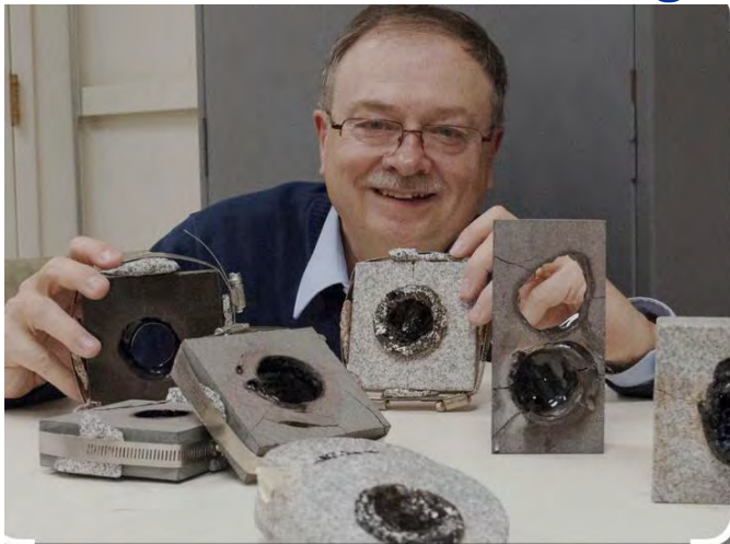
Paul Woskov at MIT: melting granite by Gyrotron beam
