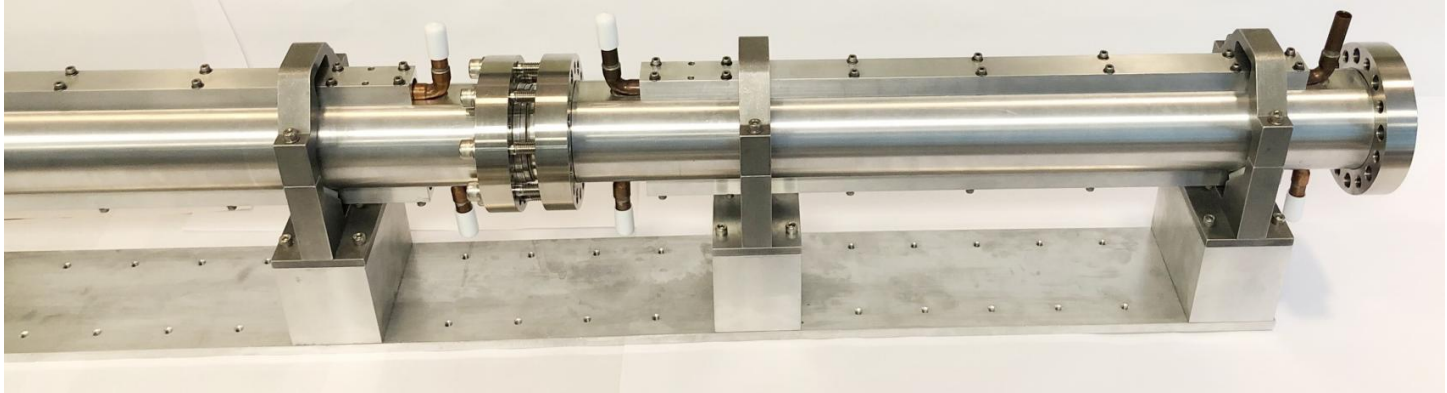
A prototype electron cyclotron transmission line assembly. Photo: US ITER
