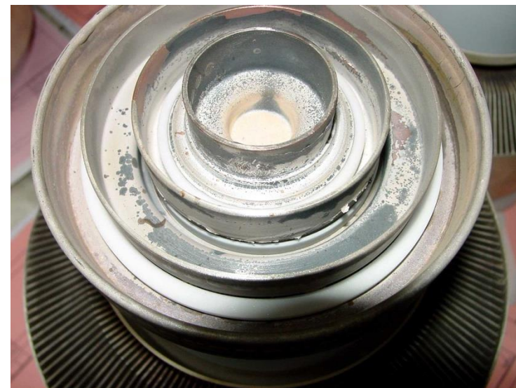
Overheating due to lack of air cooling
