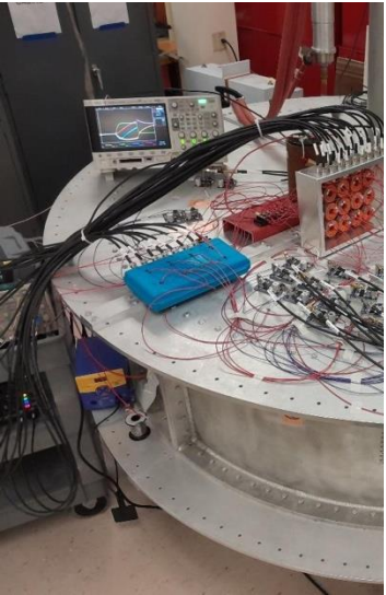
Transistor module placement in one segment of combiner top plate
