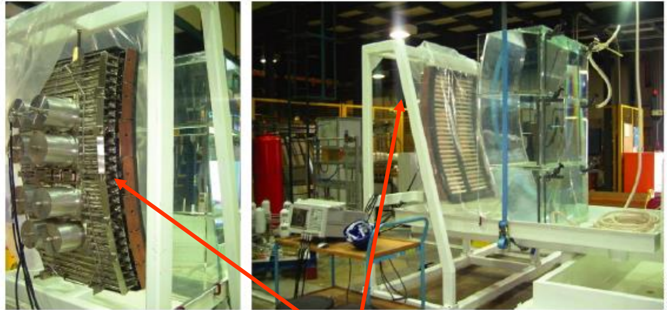
Fig. 2. (Left) Back view of the JET ITER-like antenna housing with eight attached measurement adaptors. (Right) Front view of the JET ITER-like antenna and moveable plexiglass water tank filled with salty water solution.
