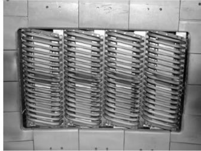
Fig. 3. One of the two newer FW antenna arrays in DIII-D. The antenna is usable over the 60- to 120-MHz band, with a self-resonance at \sim 115 MHz. The array is \sim 0.75 m wide. Here, the Faraday shield elements are bent into a U-shape perpendicular to the plane of the picture. The protective limiter surrounding the antenna is also visible.
