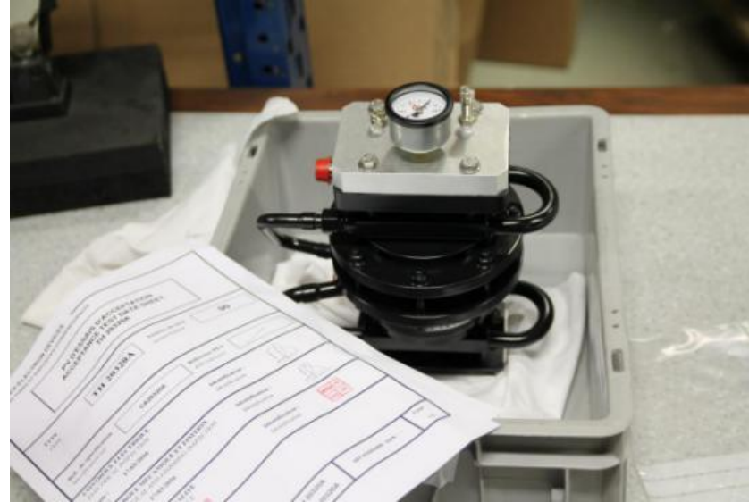
CA20320A BeO window developed by THALES, 250kW/CW
