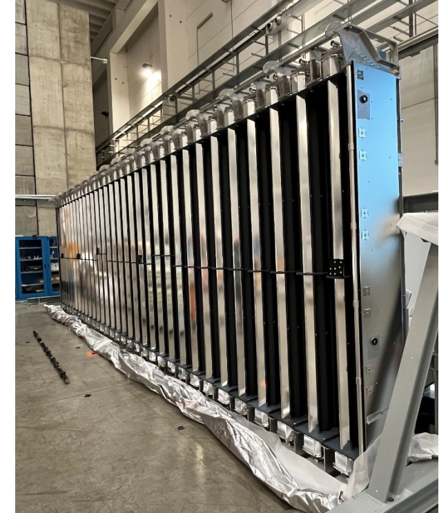
One of the two cryopanel of MITICA
