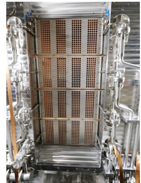
SPIDER acceleration grid with 1280 apertures
