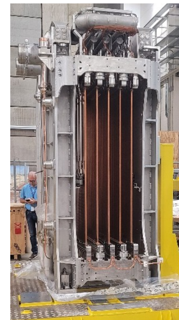
Electrostatic Residual Ion Dump and swirl-tube calorimeter in MITICA
