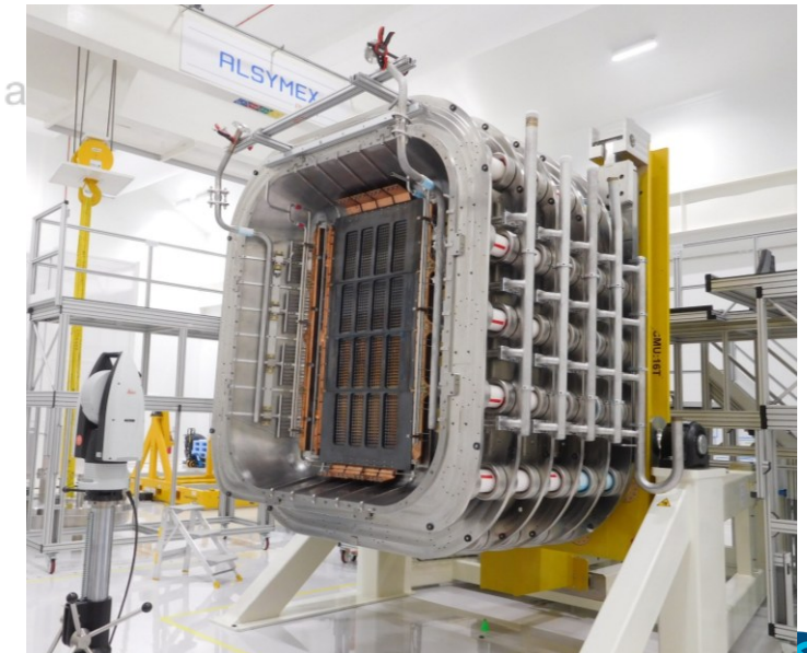
Extractor and accelerator of MITICA during alignment procedures
