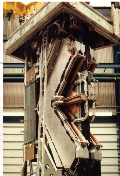
JET NB deflection magnet, residual ion dumps and calorimeter
