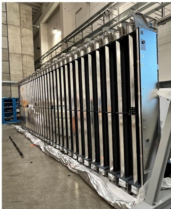
One of the two cryopanel of MITICA
