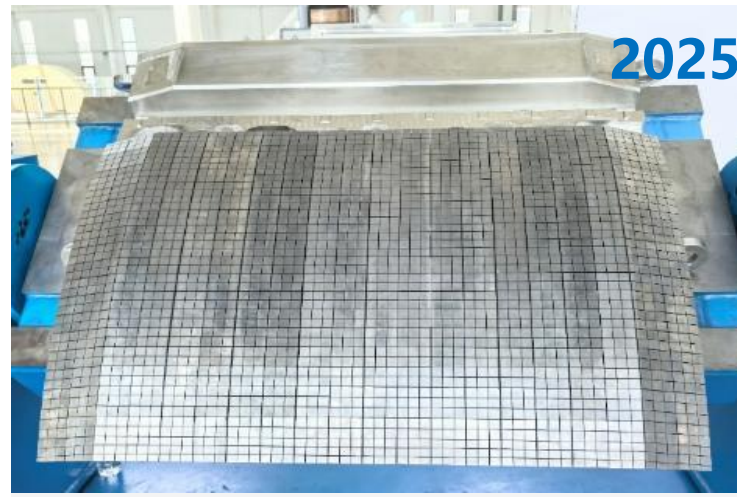
1 st Prototype of FW (tungsten armour)
