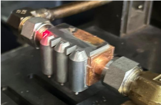
DLP under high heat load test
