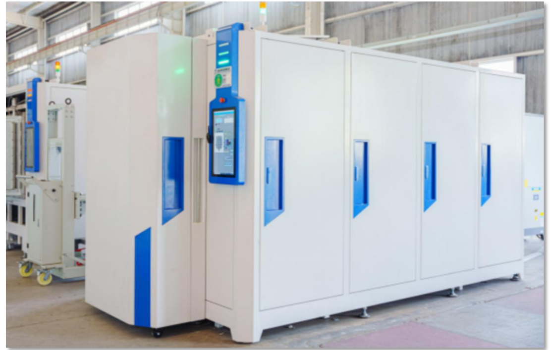
Plasma coating equipment developed by SWIP
