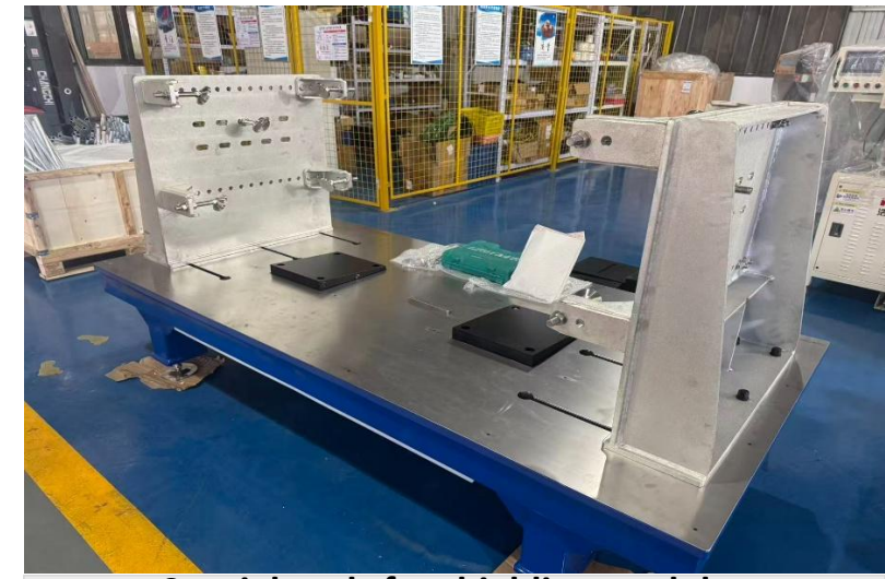
Special tools for shielding modules acceptance
