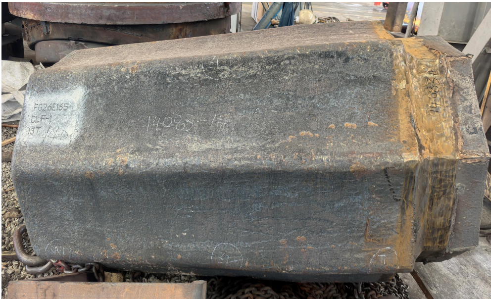
13 ton-scale CLF-1 steel ingot
