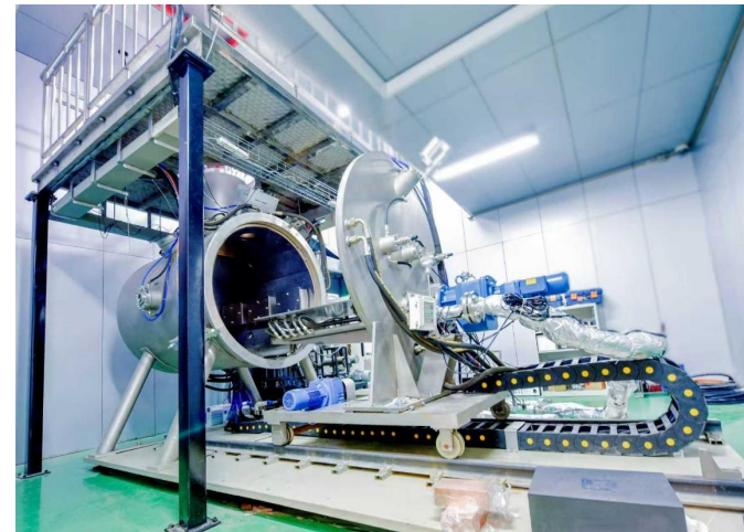
ITER-approved High Heat Load Testing platform
