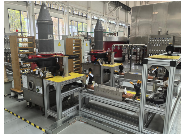
LHCD dual-tube synthesis test platform
