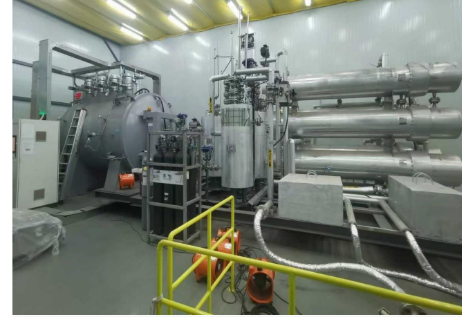
Hot Helium Leak Testing System
