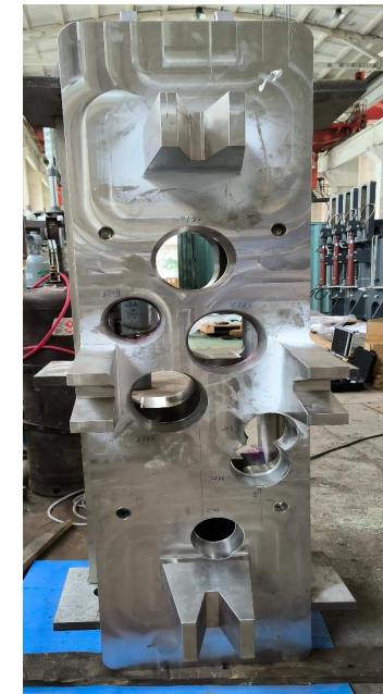
TBM Shield Block
