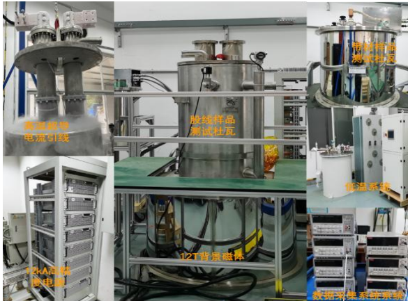
12T high field magnet (4.2K-77K, 12kA/40kA)
