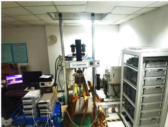
Fatigue testing machine
