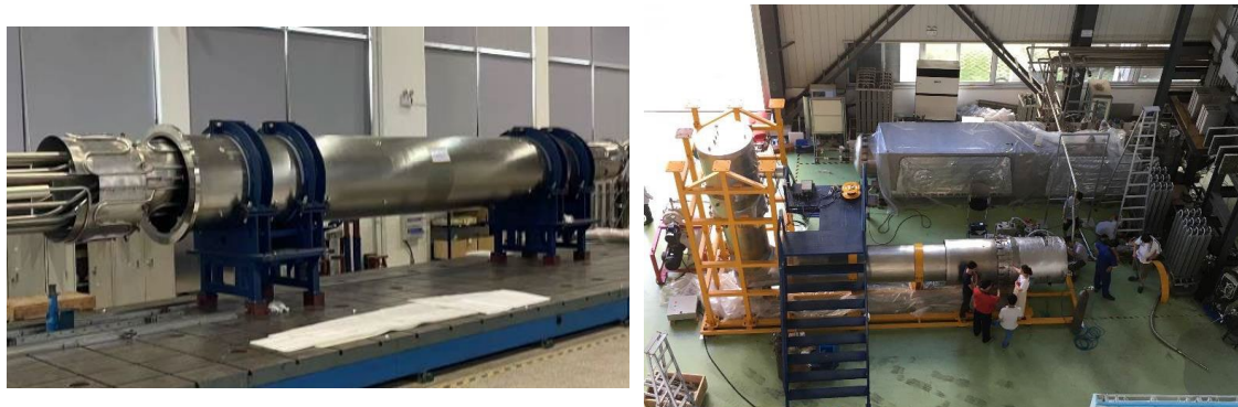
Fig. 6.1-64: Left, vacuum barrier assembly in CFT, right FAT on PF4 CFT.
