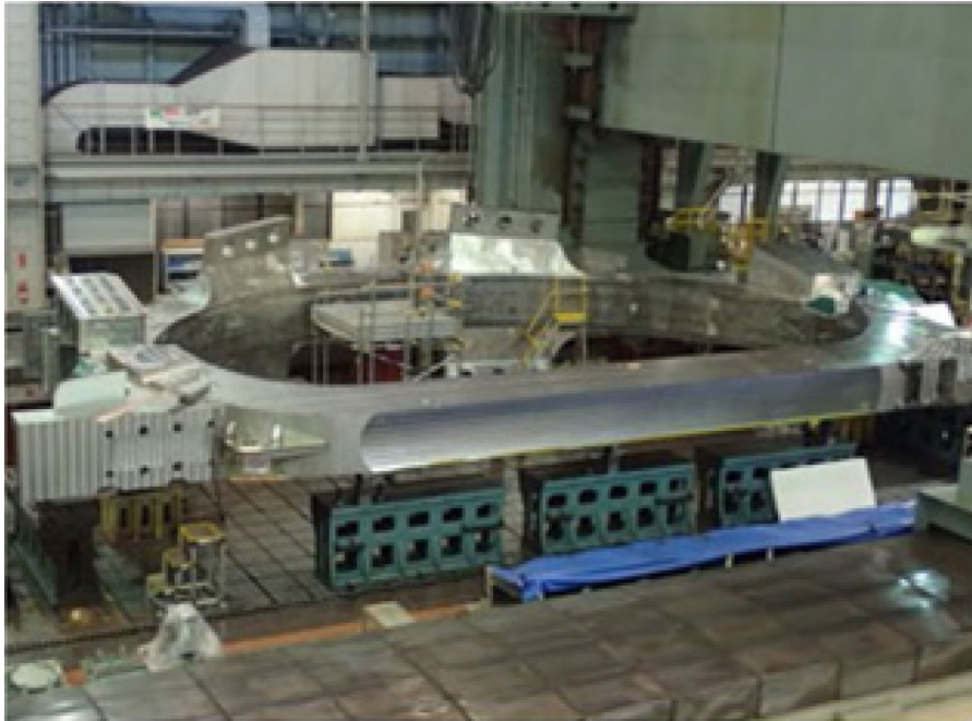
Fig. 6.1-75: TF coil on the Super Miller at MHI
