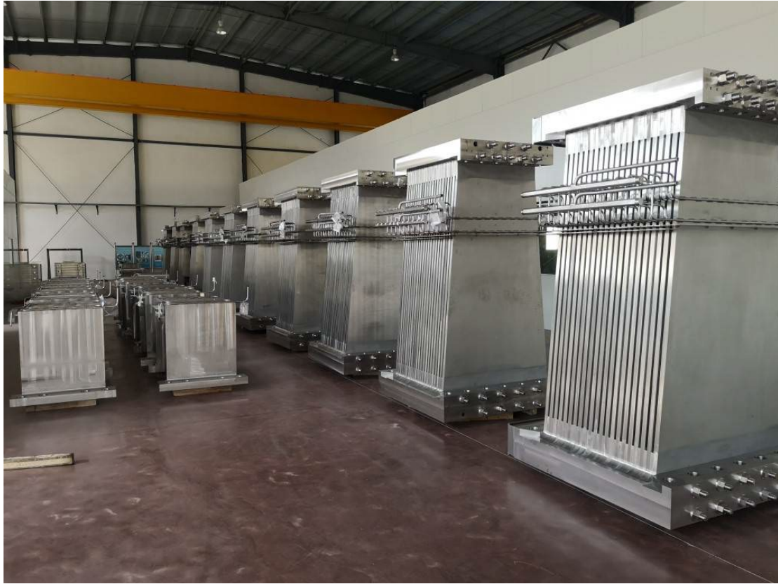
Fig. 6.1-55: Completed TFGS Gravity Supports (right) and PF Supports (left)
