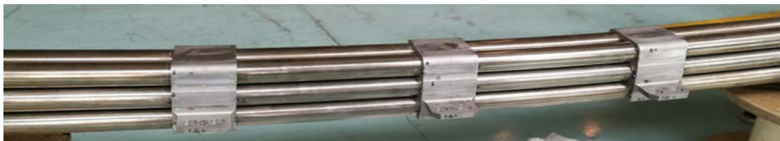
Fig. 6.1-66: Top, IVC Conductor, Bottom Supports welded to ELM coil conductors.
