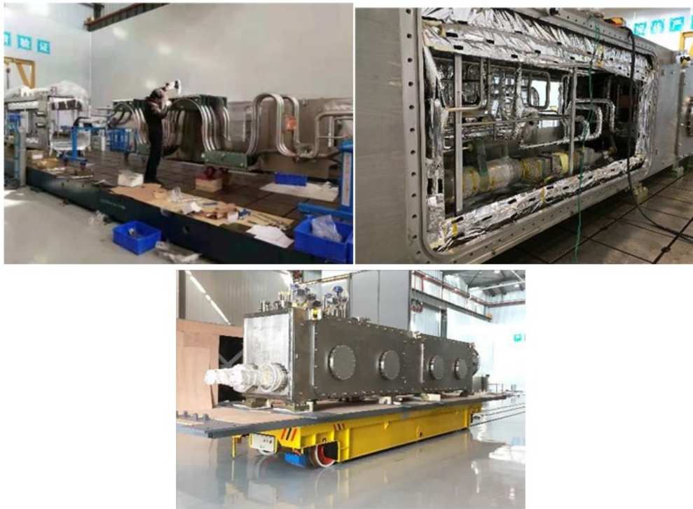
Fig. 6.1-63: Feeder Component Manufacture Ongoing (left, S-bends, middle CTB internal pipes and current leads, right completed CTP).
