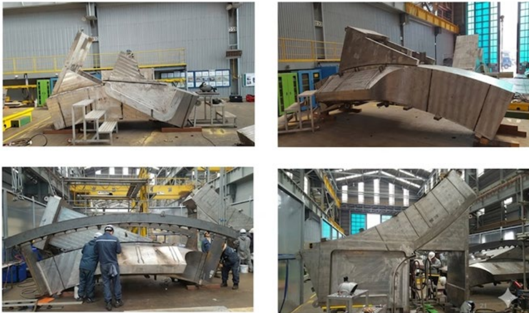
Fig. 6.1-73: Main TF Case Segments under Manufacture.
