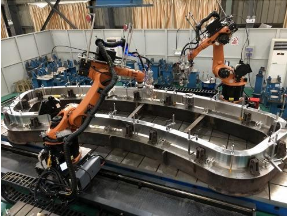
Fig. 6.1-62: Bottom correction coil, case closure welding.
