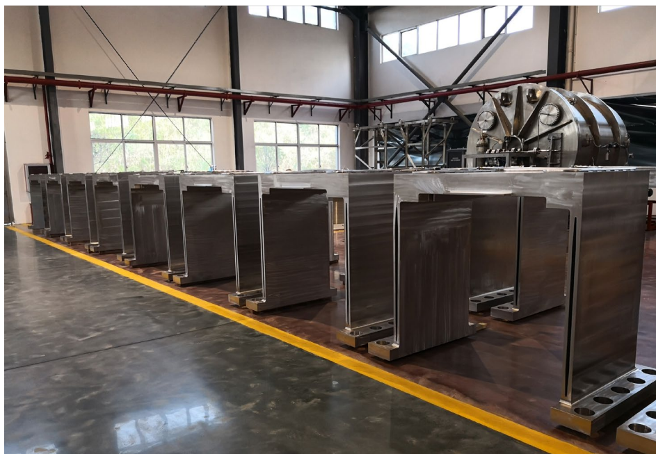
Fig. 6.1-58: PF Structures (flexible supports) Under Manufacture at HTXL.
