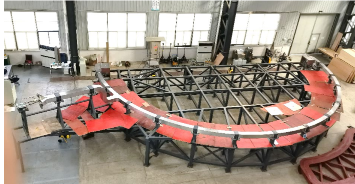
Fig. 6.1-65: Correction Coil in Cryostat Feeder.
