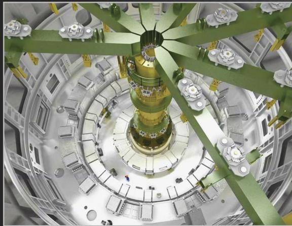
The In-Pit Assembly tool is made up of a central tower and a series of beams. This tool will support the vacuum vessel sub-assemblies (three groups of three sectors) and align them while the vacuum vessel is welded together.
