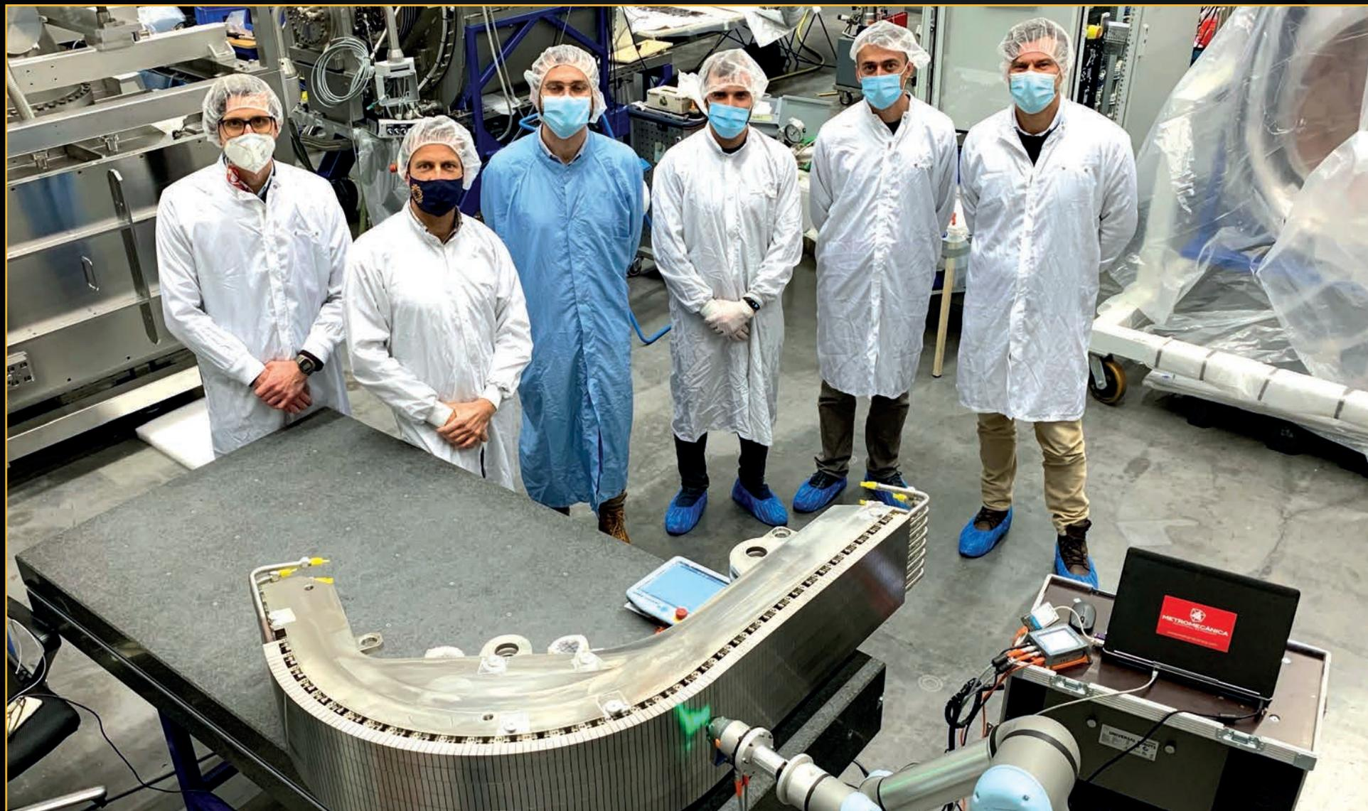
Representatives of Fusion for Energy (F4E), Research Instruments, and Metromecanica observe dimensional tests on a full-scale divertor inner vertical target prototype. The target's surface is made of small monoblocks in tungsten, which can withstand some of the highest heat loads of the ITER machine.
