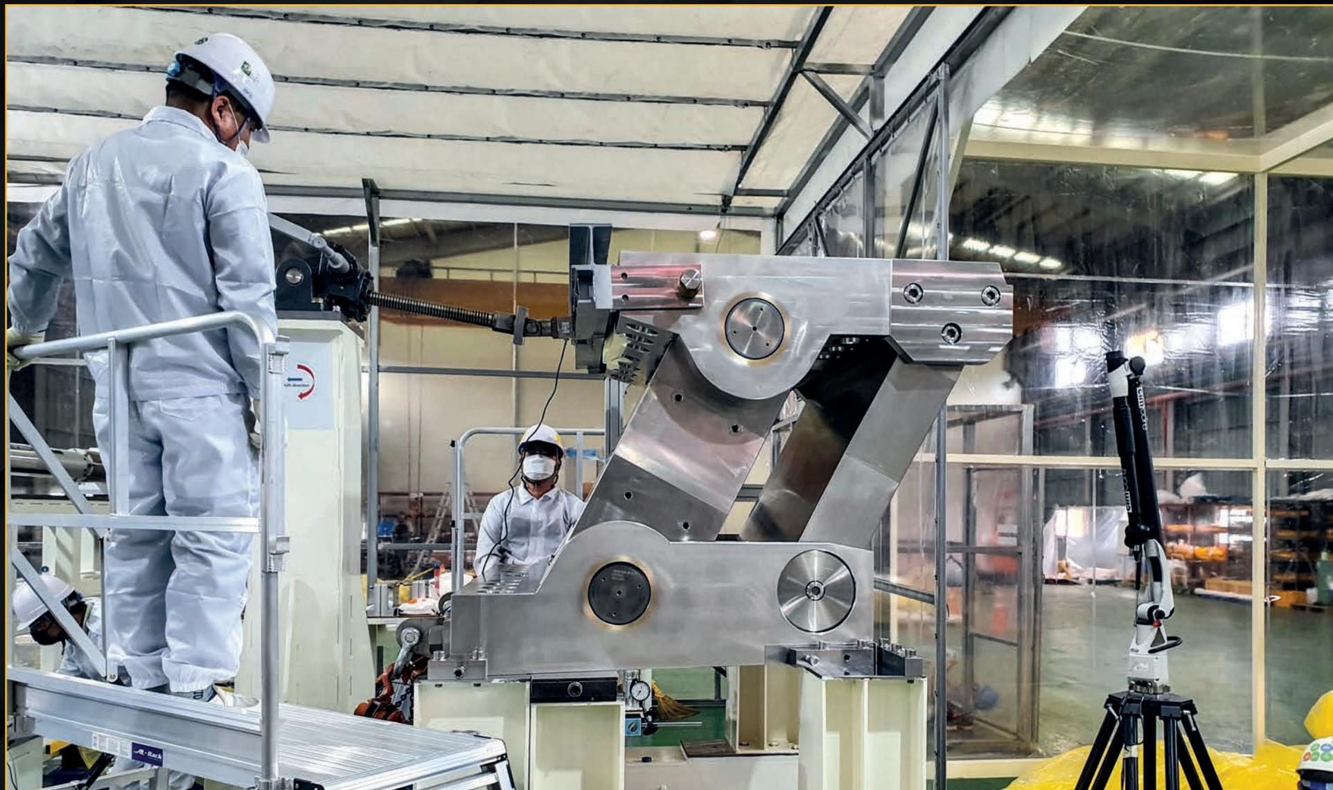
The factory acceptance test on the first ITER vacuum vessel gravity support has been successfully completed at Haneul Engineering in Gunsan, Korea. Under the plasma chamber, nine gravity supports will allow for the vacuum vessel's thermal expansion and sustain loads in the radial, toroidal and vertical directions.
