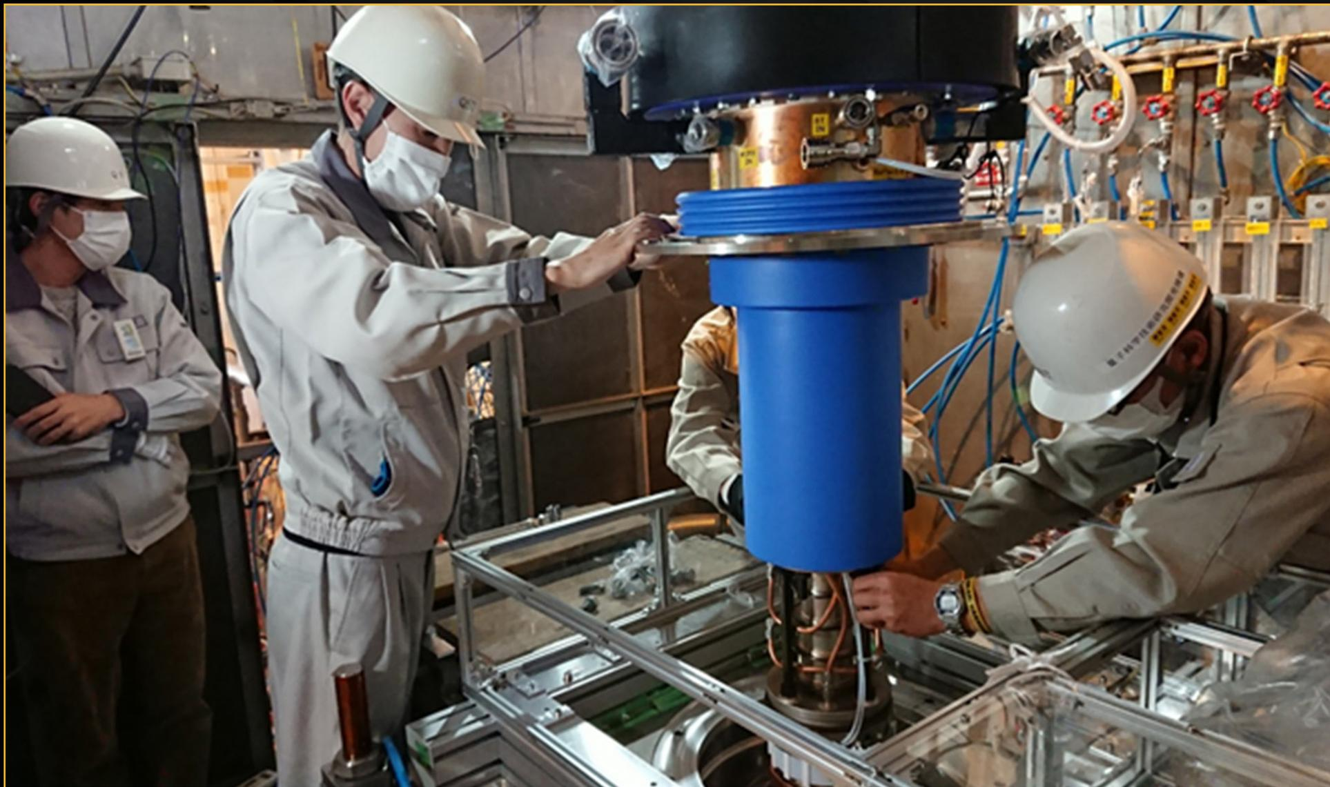
A gyrotron is carefully inserted into the narrow bore of a superconducting magnet. The technicians lower the gyrotron with a crane slowly to minimize vibrations.
