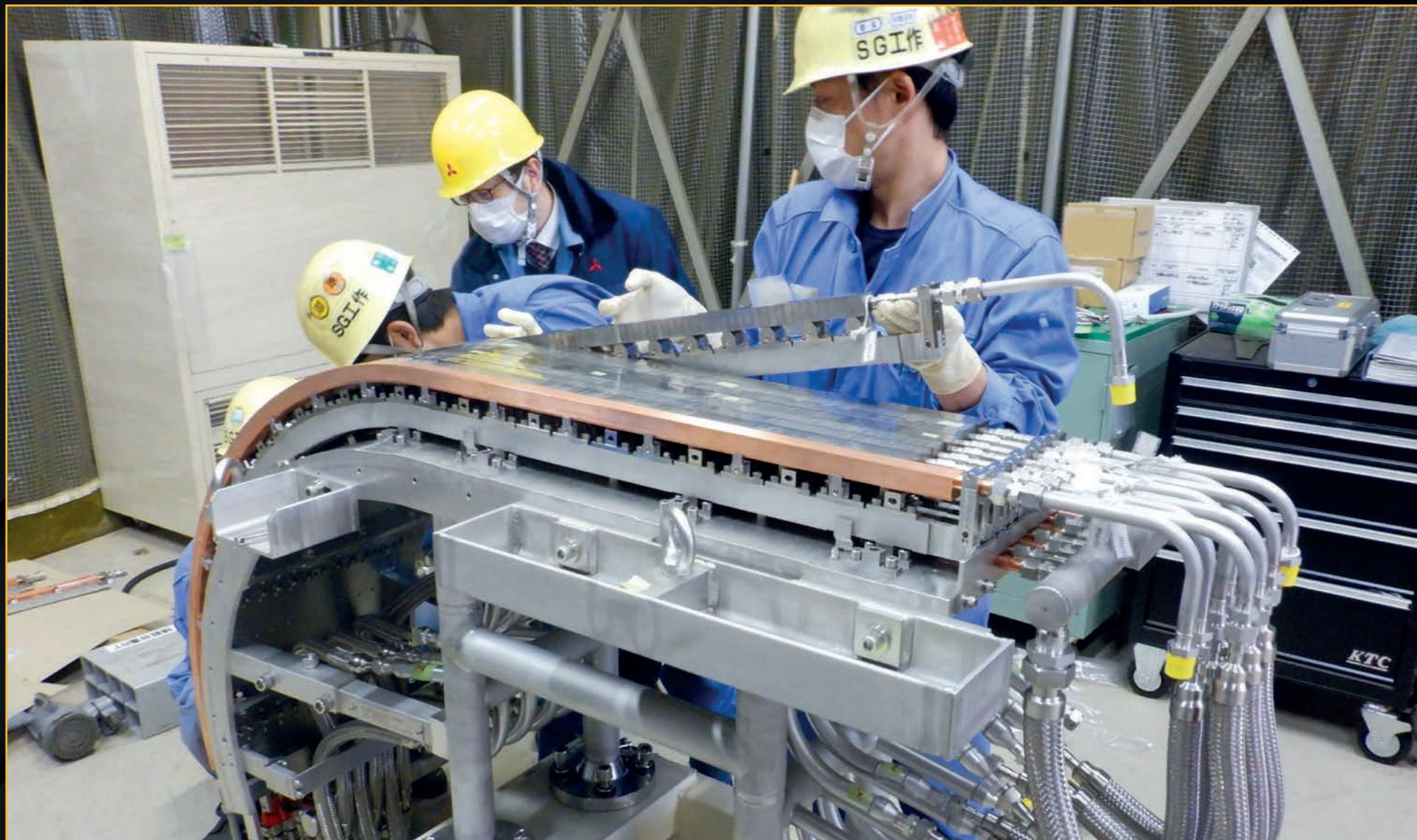
Plasma-facing units of the ITER divertor outer vertical target prototype have been mounted on a test assembly for high heat flux heating. The conditions at the bottom of the machine, where waste gas and impurities are exhausted from the reactor, can be described as "extreme."
