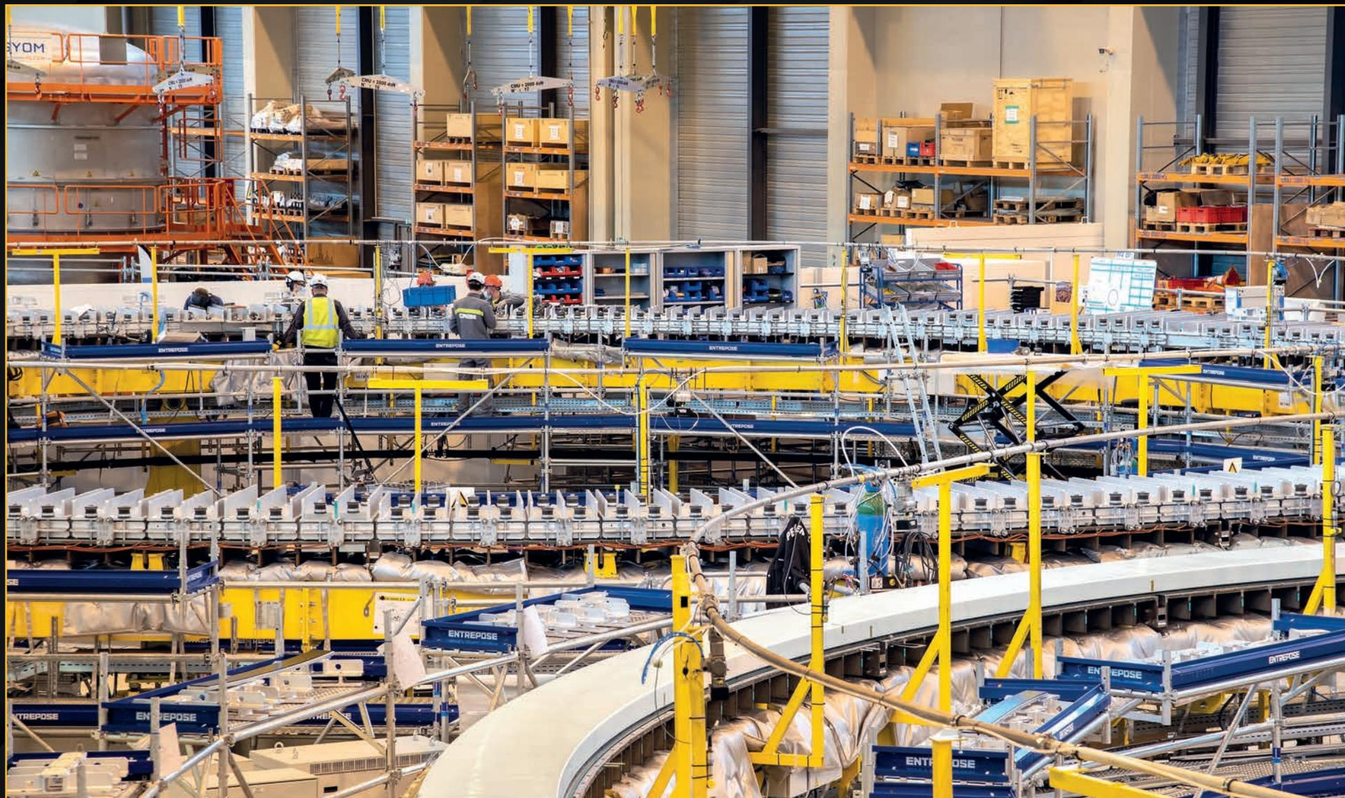
In its on-site winding facility, the European Domestic Agency Fusion for Energy (F4E) is producing four poloidal field coils. Each one is formed by stacking layers of conductor called double pancakes, pictured here in production. **January 2021**
