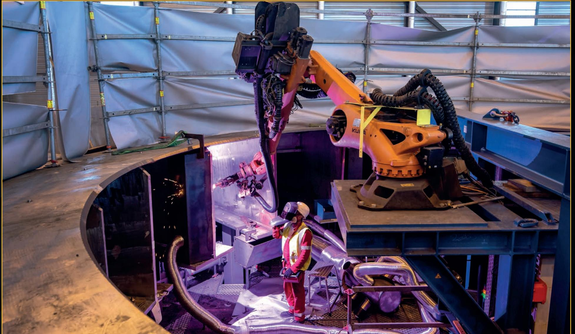
Of the four sections that make up the ITER cryostat, the top lid is the thickest, second heaviest (665 tonnes) and most structurally complex. The component is finalized by Indian Domestic Agency contractors in March 2022 and handed over to the ITER Organization. **September 2021**
