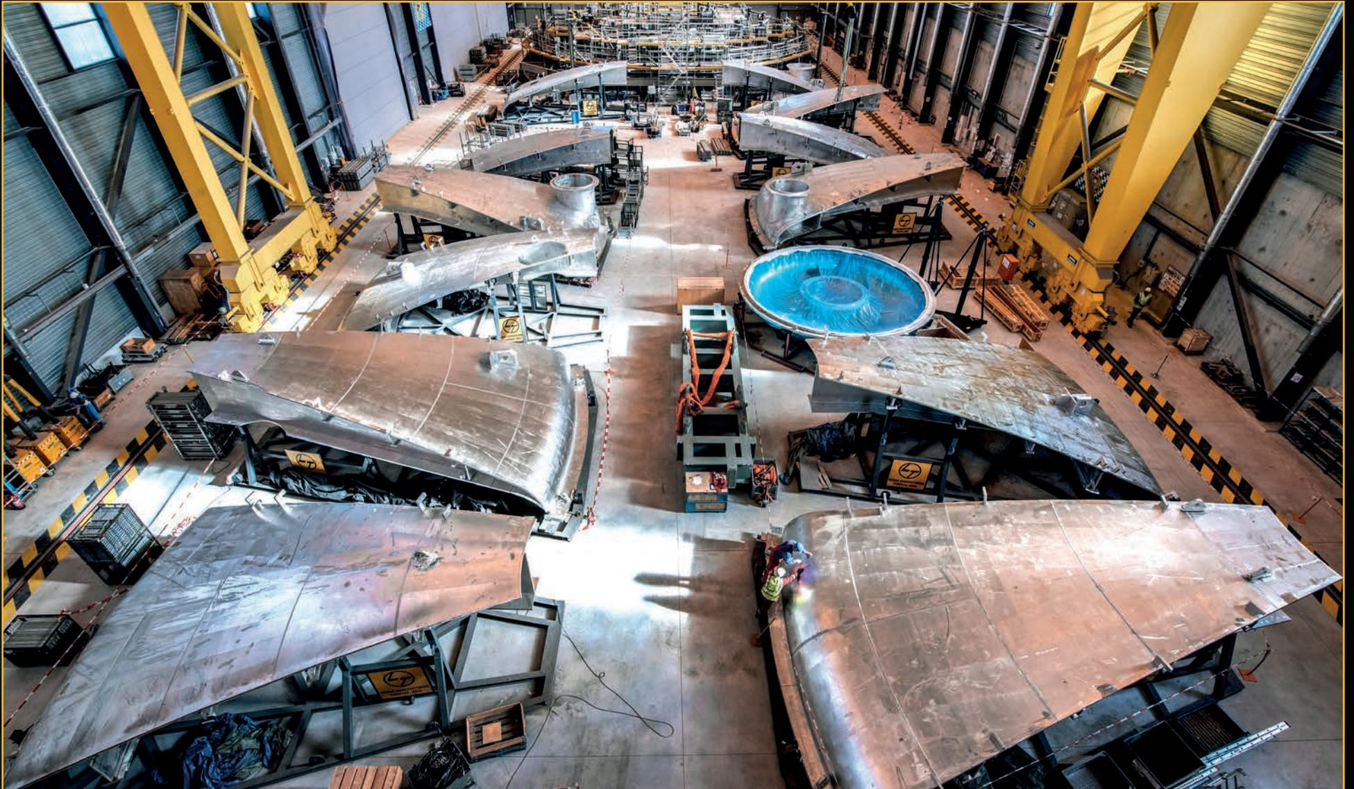
The segments of the cryostat lid arrive early in the year from India. They will be aligned and welded on the platform at the far end of the Cryostat Workshop. **February 2021**
