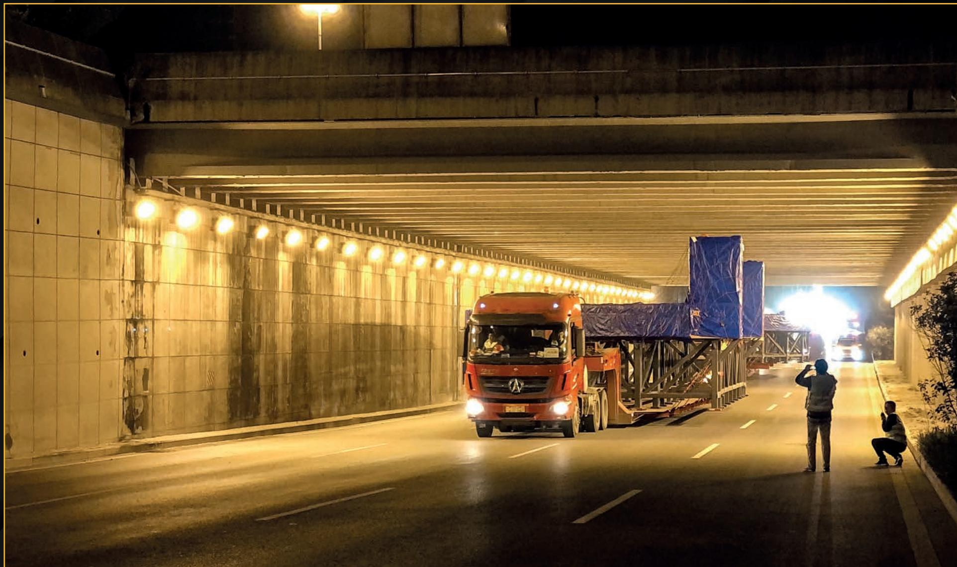
Semi-circular magnet feeder elements are travelling from the Institute of Plasma Physics (ASIPP) in Hefei to the nearest port for shipment to ITER. China is providing approximately 1,600 tonnes of feeder segments, or 100 large components.
