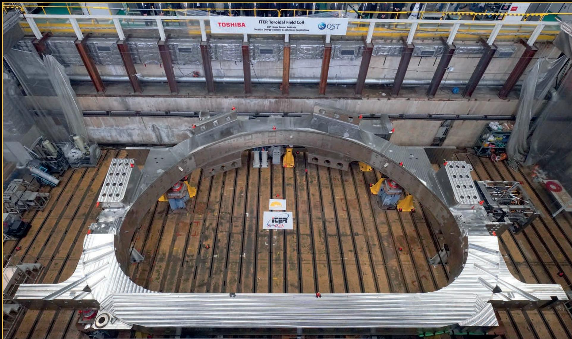
In June 2021, Toshiba Energy Systems & Solutions produces the first of four ITER toroidal field coils on behalf of Japan's QST\*, the National Institutes for Quantum and Radiological Science and Technology. QST is supplying 9 toroidal field coils (winding packs and coil structures) plus another 10 coil structures to the ITER Project
