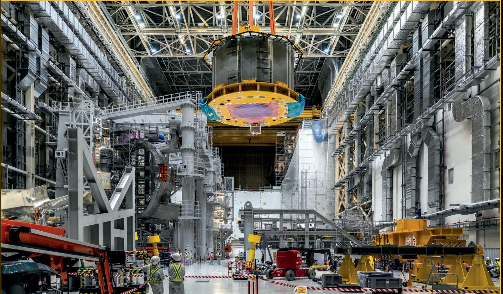
The first of six central solenoid modules is transferred to a staging area in the Assembly Hall. Six modules will be stacked to form the 1,000-tonne central magnet of the ITER machine. **February 2022**
