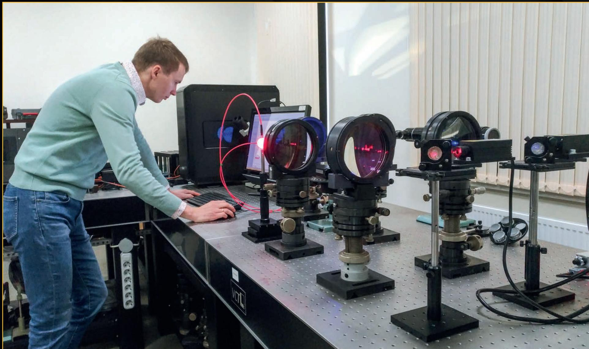
At a spectroscopic laboratory in Moscow, Russian Domestic Agency specialists are working to support the development of optical diagnostic systems for ITER, such as the Charge eXchange Recombination Spectroscopy (CXRS) Edge diagnostic.
