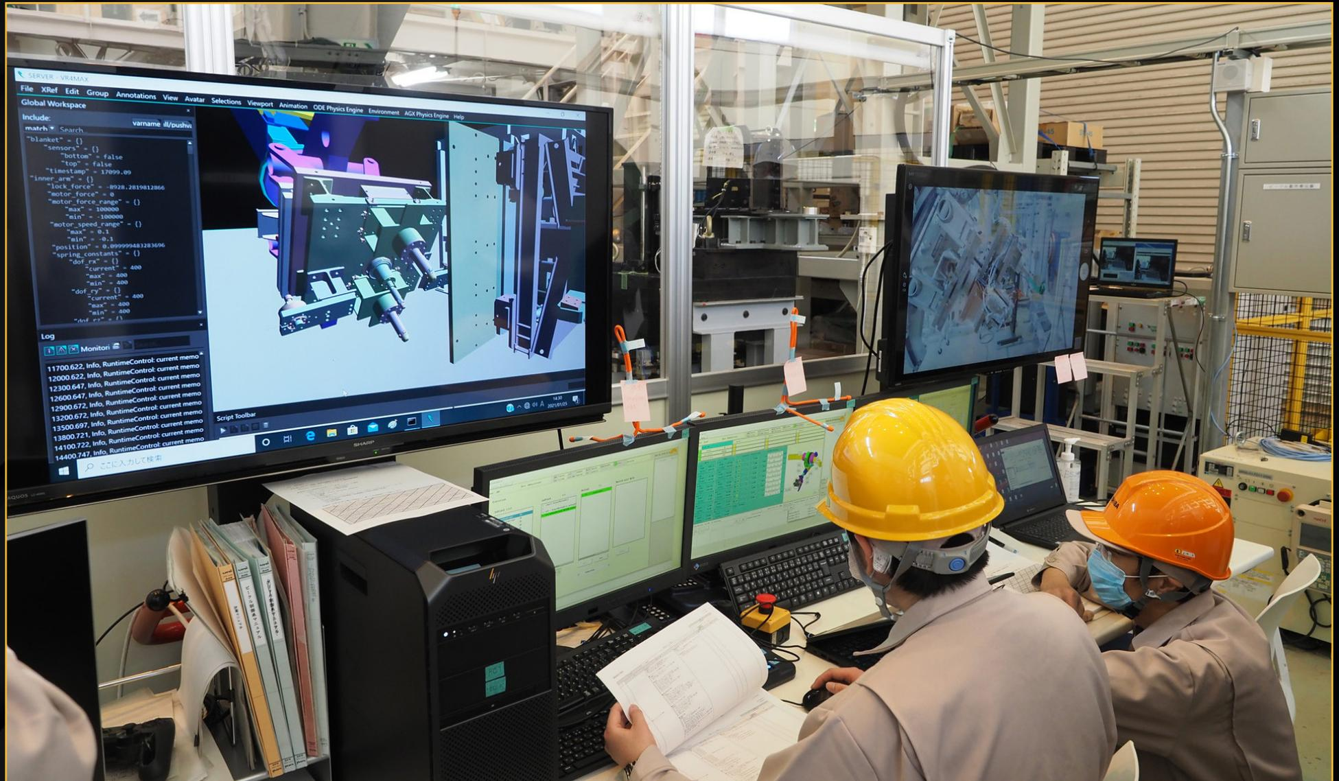
Engineers test a prototype of the control system for the ITER blanket remote handling system. On the left screen is a virtual reality model, on the right screen is the view from the camera. If you look closely you can spot the manipulator that is being controlled behind the screen.
