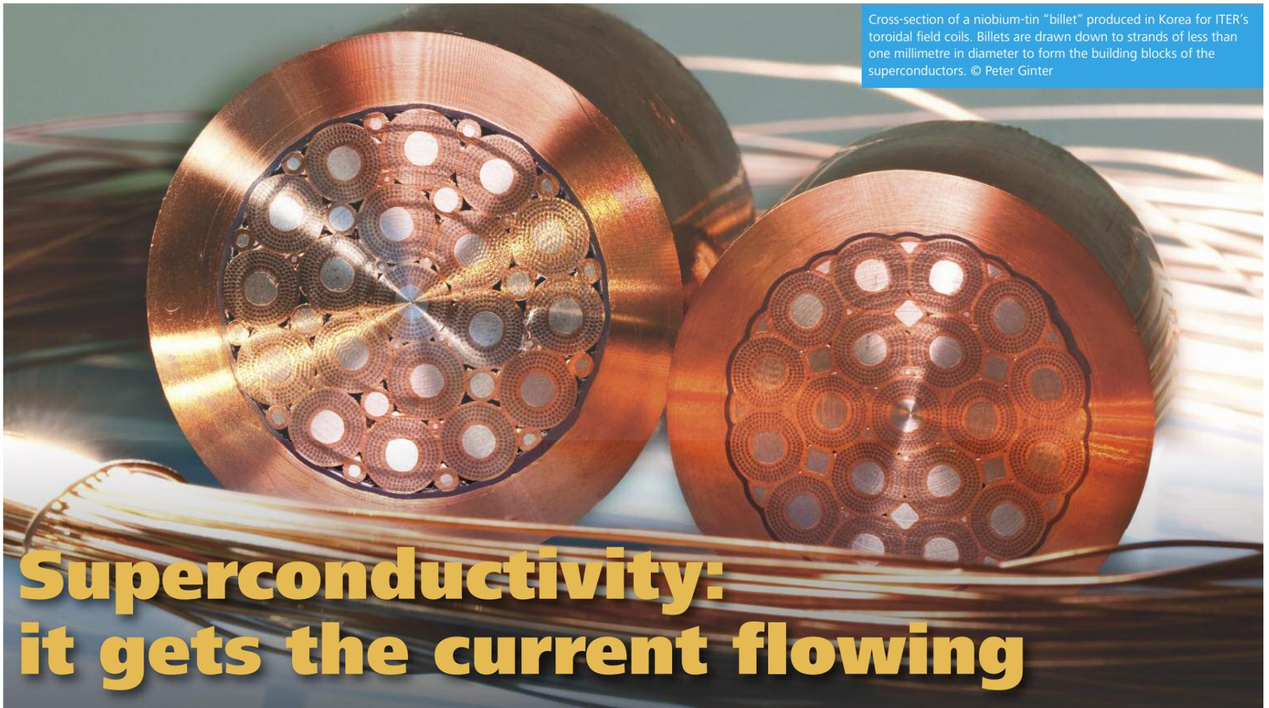
Cross-section of a niobium-tin "billet" produced in Korea for ITER's toroidal field coils. Billets are drawn down to strands of less than one millimetre in diameter to form the building blocks of the superconductors. © Peter Ginter
