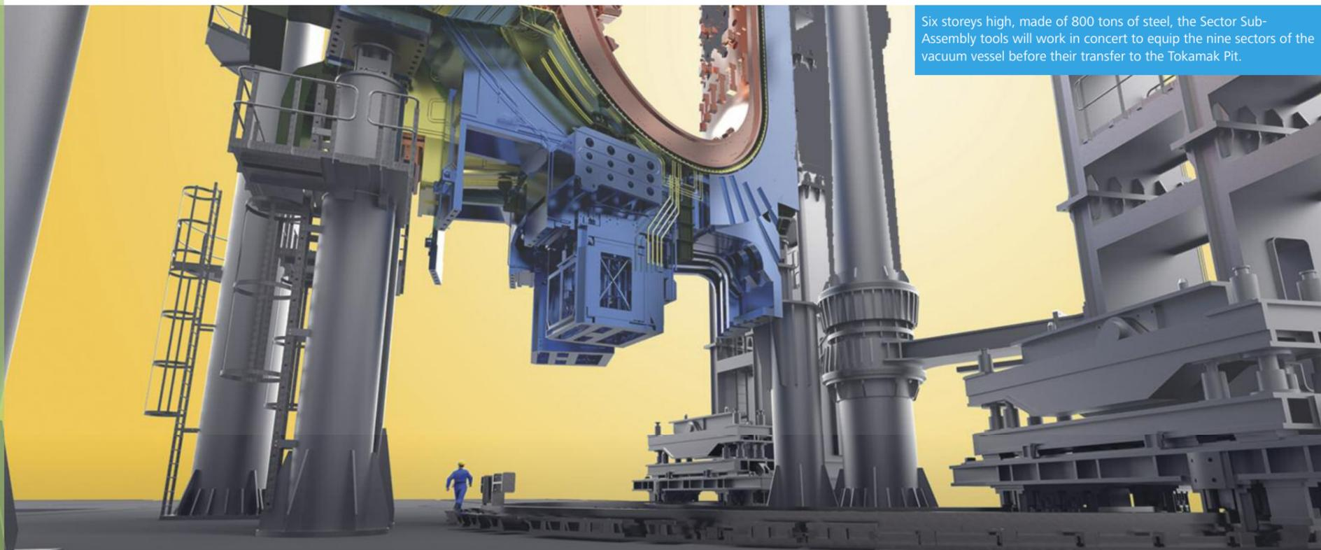
Six storeys high, made of 800 tons of steel, the Sector Sub-Assembly tools will work in concert to equip the nine sectors of the vacuum vessel before their transfer to the Tokamak Pit.
