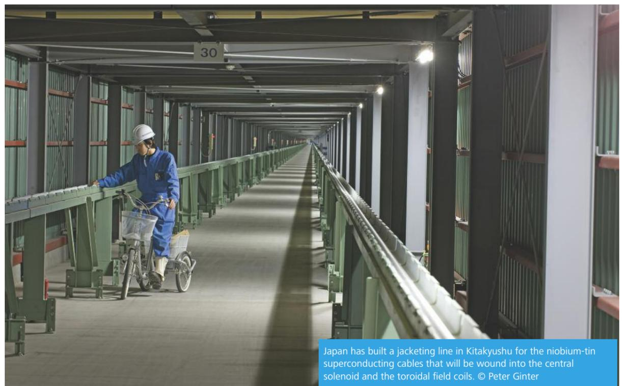
Japan has built a jacketing line in Kitakyushu for the niobium-tin superconducting cables that will be wound into the central solenoid and the toroidal field coils. © Peter Ginter
