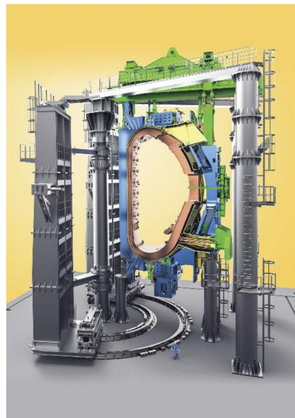
Standing shoulder to shoulder, two Sector Sub-Assembly tools will suspend the vacuum vessel sectors from the top while carefully positioning and installing – via the rotary motion of the "wings" – the vacuum vessel thermal shielding and two toroidal field coils.
