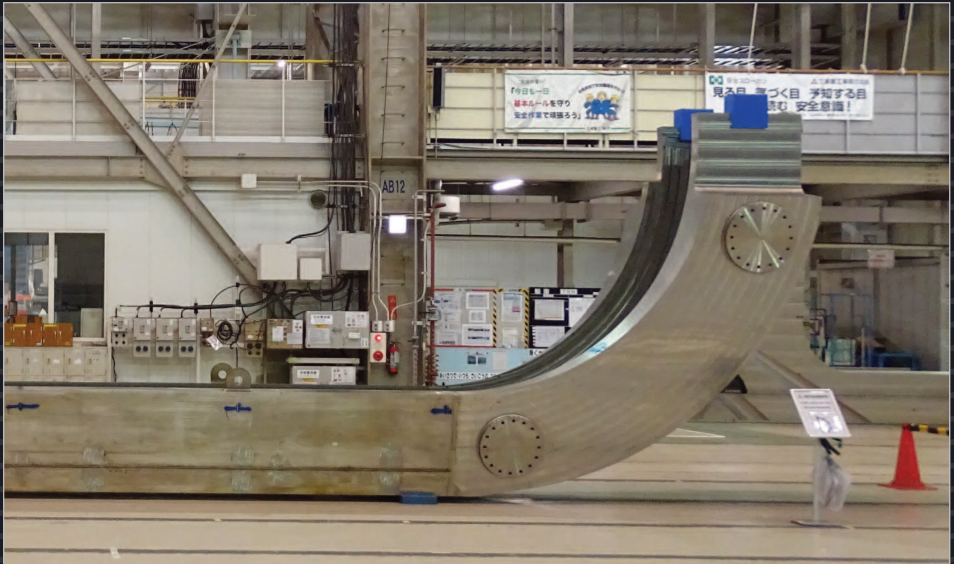
Connection of segments for the first inboard TF structure was completed in November 2015, marking a significant achievement of milestone for TF coil procurement.
