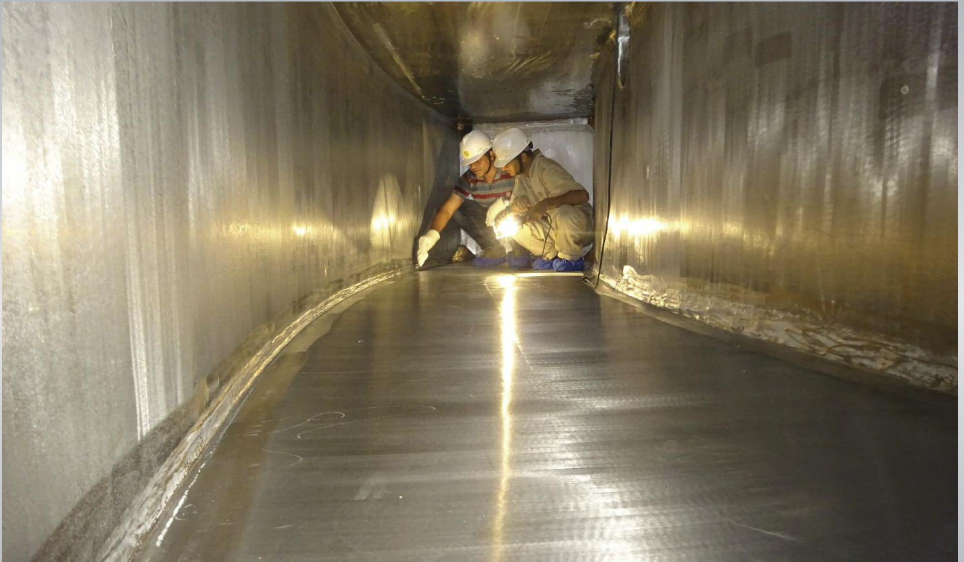
In the cryostat manufacturing facility in India, a segment of the pedestal ring (part of tier 2 of the base) is inspected before delivery to ITER. Responsible for the manufacturing design, fabrication and assembly of the 3,850-tonne ITER cryostat, India is shipping the cryostat to ITER in 54 segments for on-site assembly.
