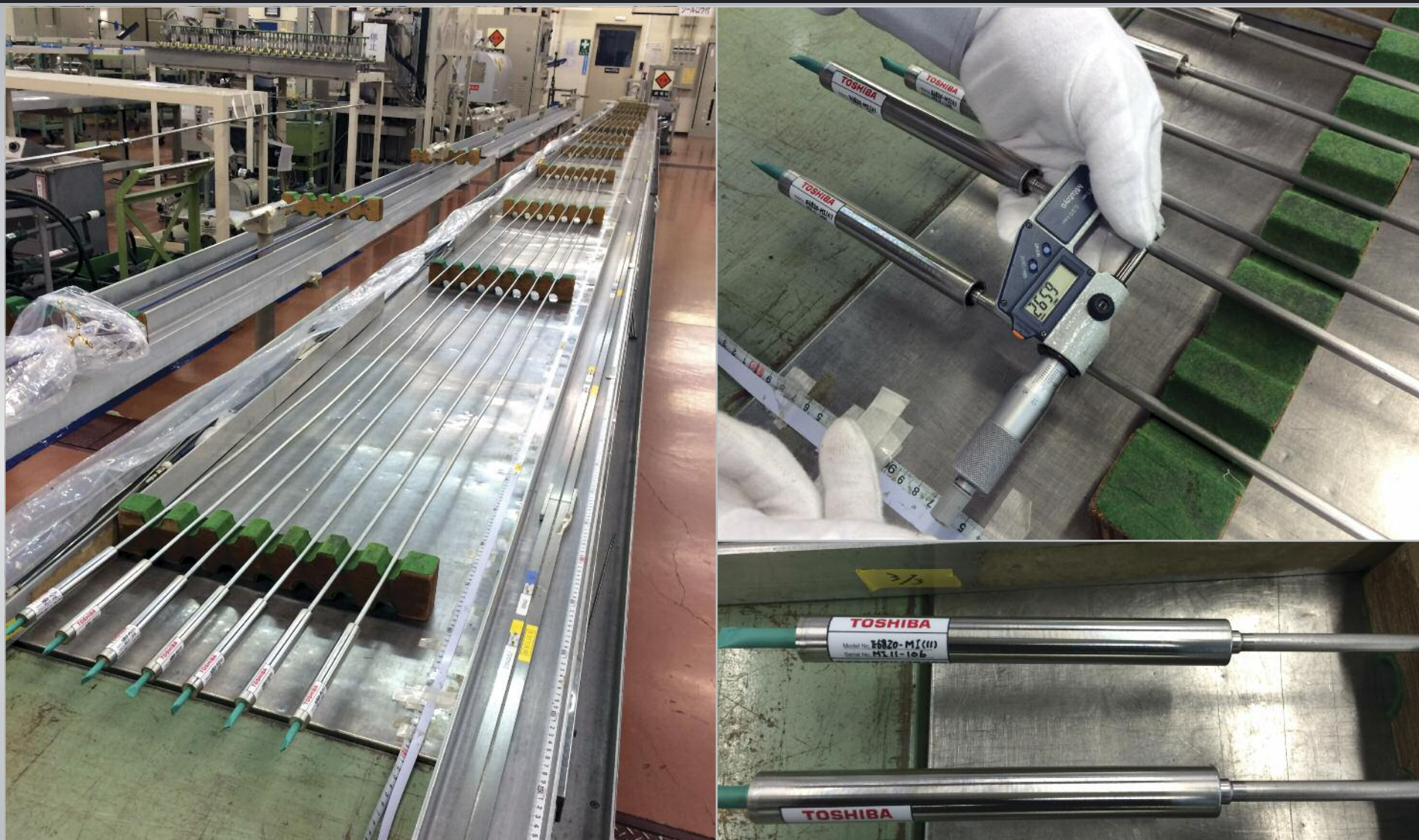
Mineral insulated (MI) cables have been manufactured by Toshiba Co Ltd under contract with QST. These MI cables will deliver signals from micro fission chambers which are located near the plasma to “count” neutrons during operation as a way to measure fusion power.
