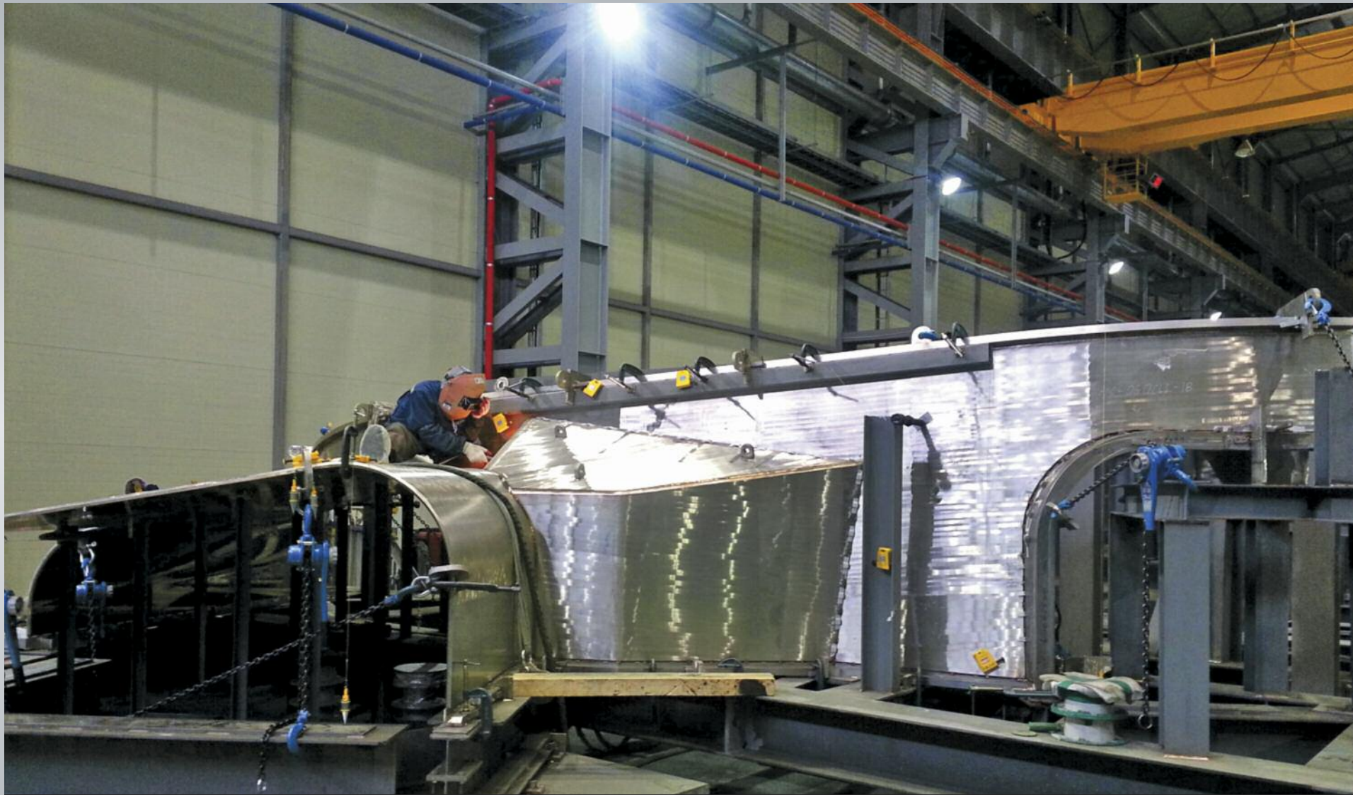
A thin barrier of stainless steel (10-20 mm), actively cooled and covered with a low-emissivity coating of silver, will protect the magnet coils from thermal radiation. At SFA Engineering in Changwon, welding is underway on an outboard sector of the vacuum vessel thermal shield.
