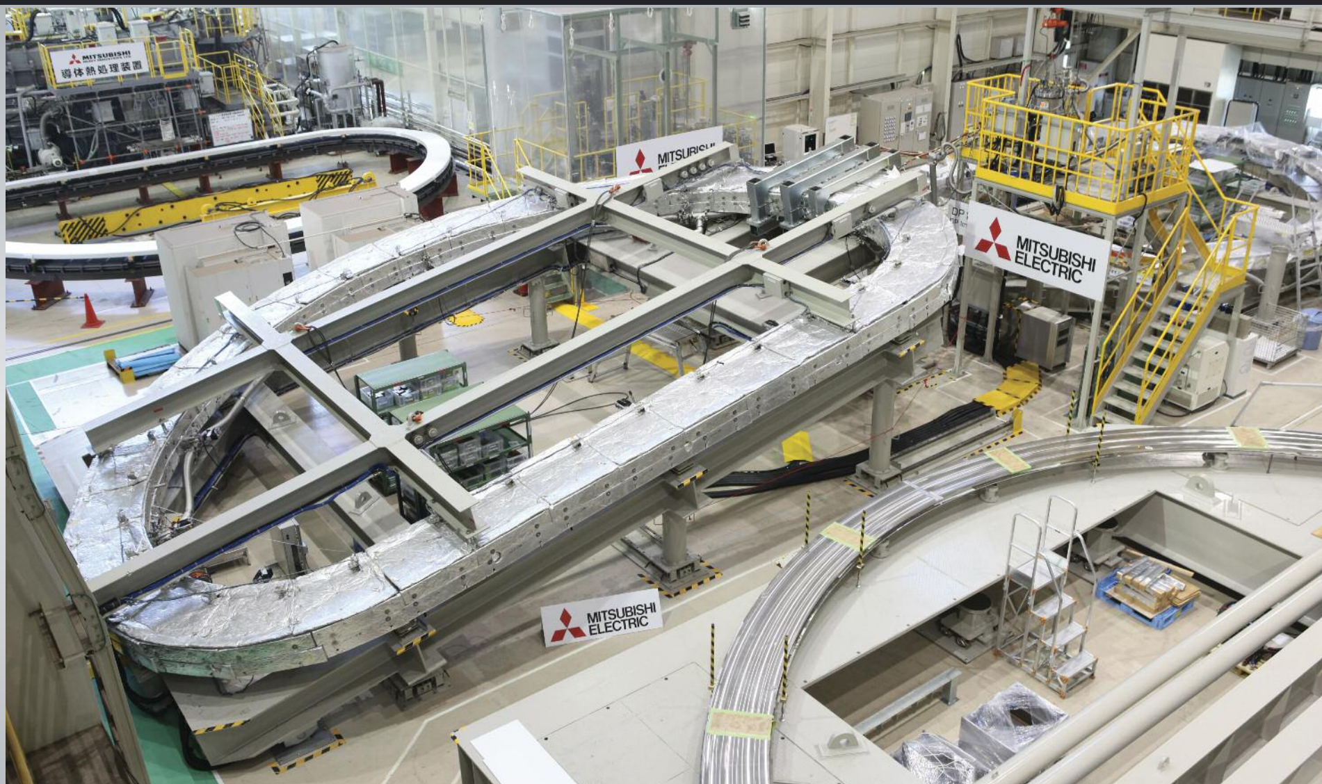
Toroidal field coil windings are first insulated with glass and polyimide tape, then impregnated with cyanate-ester and epoxy resins to harden the assembly. Thirty-five double-pancakes – the building blocks of the toroidal field coils – have been insulated and impregnated at Mitsubishi Heavy Industry's Futami factory.
