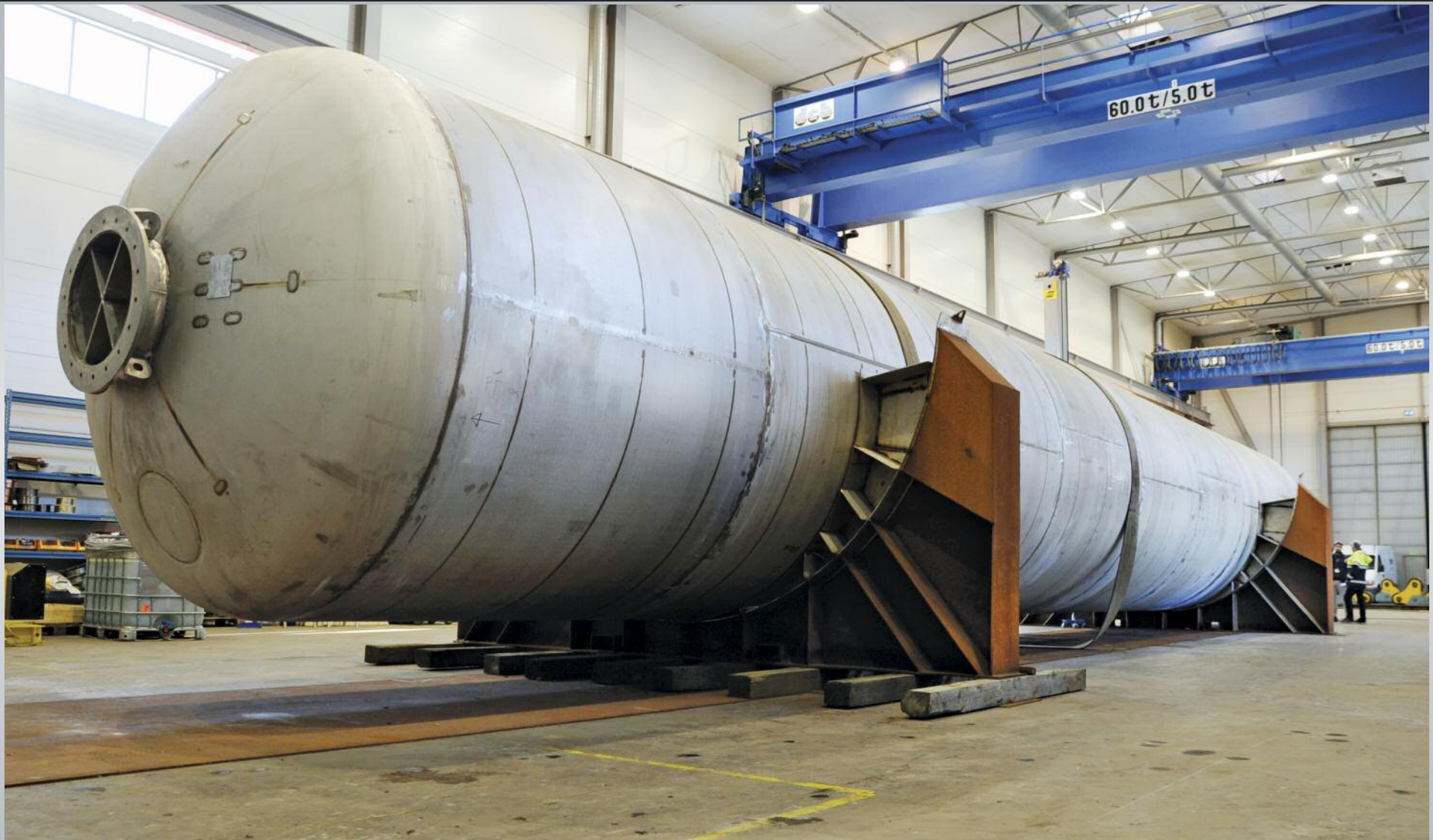
A 23-metre storage tank for liquid helium, part of Europe's contribution to ITER's liquid nitrogen plant and auxiliary systems, has successfully passed leak tests. The 190 m 3 stainless-steel tank will store liquid helium at -269 °C.
