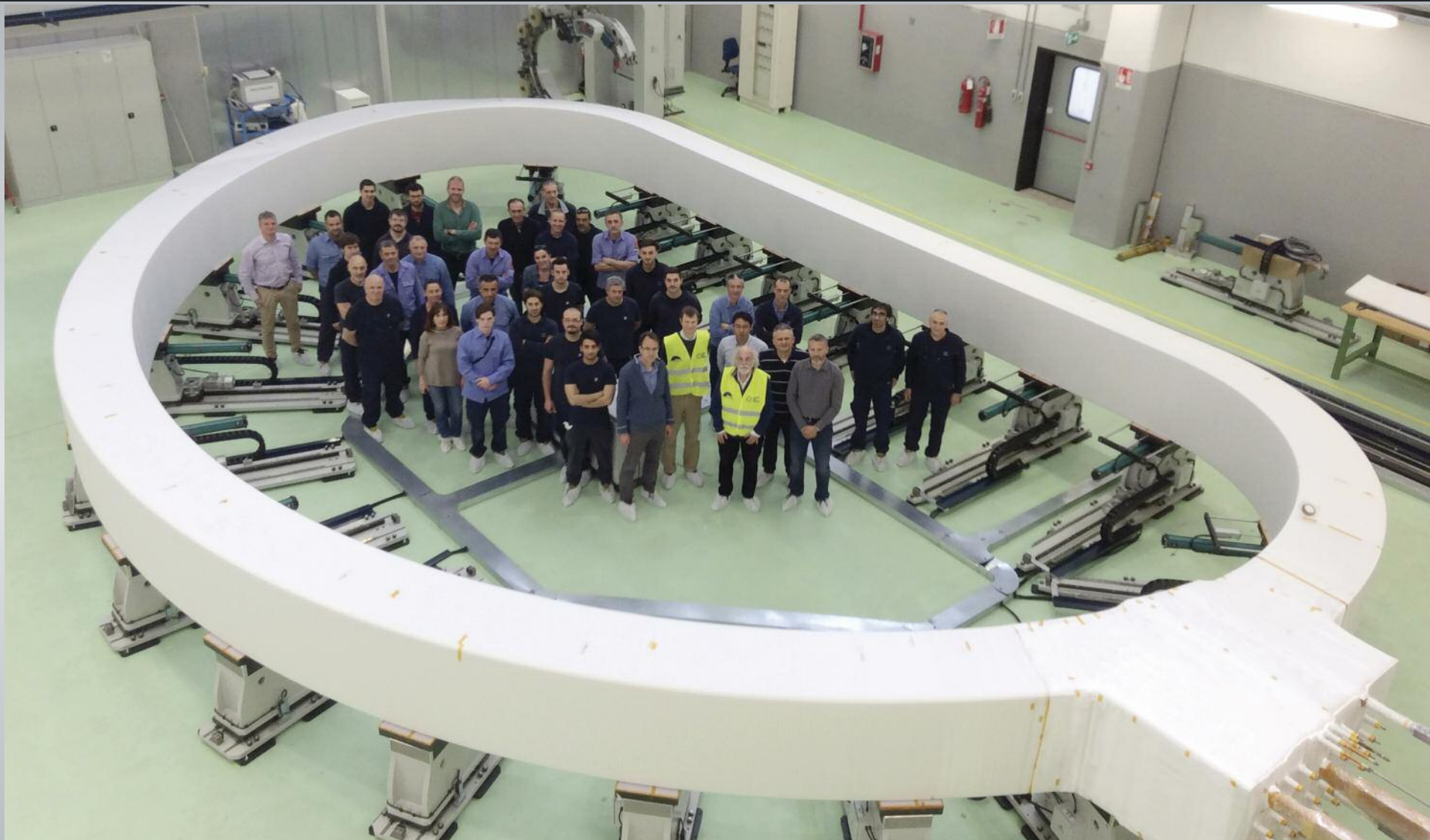
D-shaped toroidal field coils will create the magnetic field that confines the ITER plasma. In 2016, the first toroidal field “inner core” – called a winding pack – is successfully produced in Europe. Following testing, it will be inserted into a stainless steel coil case to form the final 310-tonne coil assembly.
