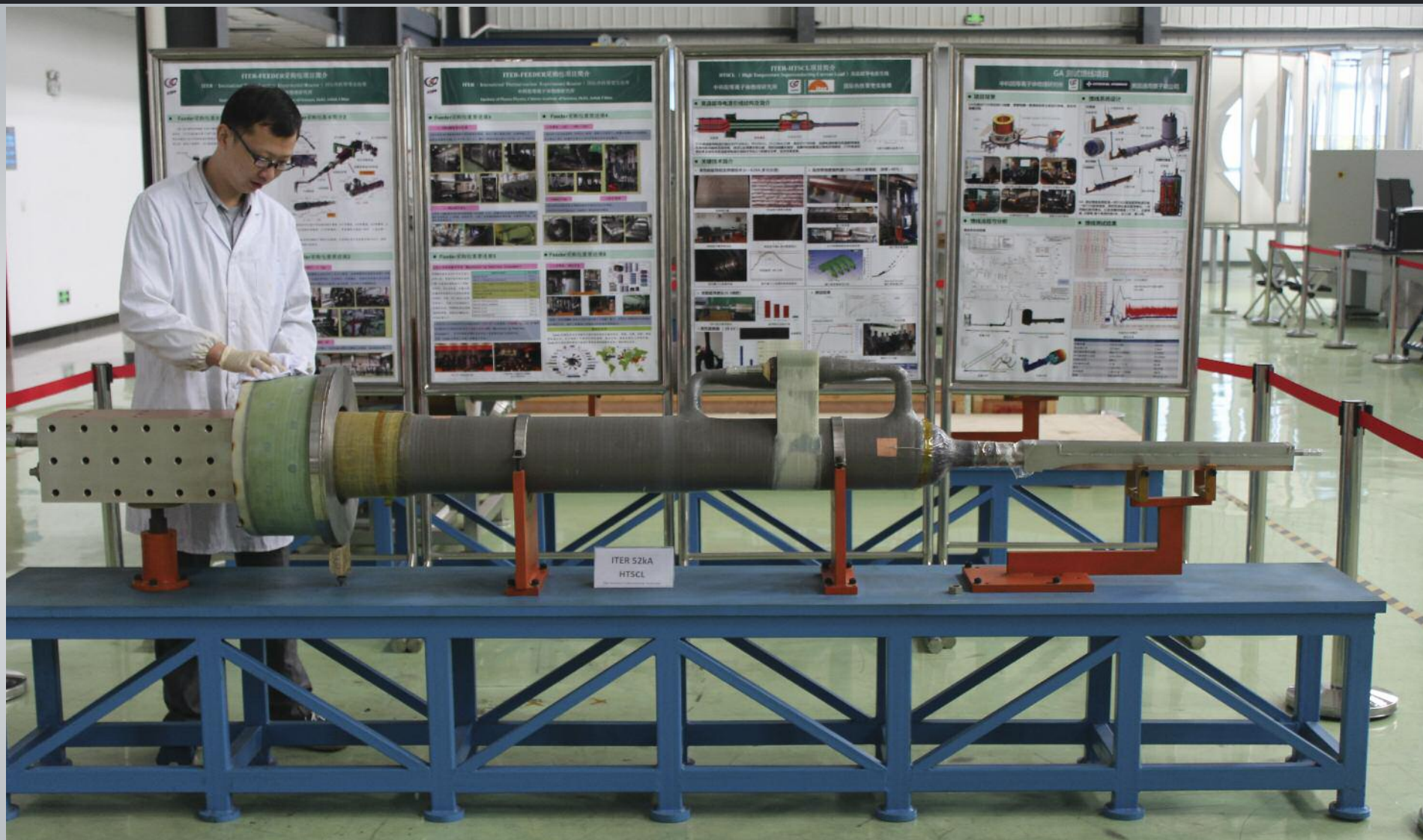
High temperature superconductor (HTS) current leads will transfer large amounts of current from room-temperature power supplies to very low-temperature superconducting magnets. The 52 kA current lead prototype pictured (poloidal field and central solenoid type) has been successfully tested at ASIPP.
