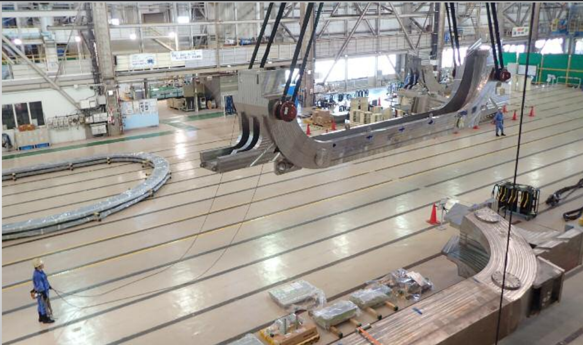
The inboard side structures for the ITER TF coil cases are now in series production at the Futami Plant of Mitsubishi Heavy Industries, Ltd.. The inboard side structures consist of a single long straight section in the center, and two curved parts at both ends. They are made of a special austenitic stainless steel and measure 16 m long.
