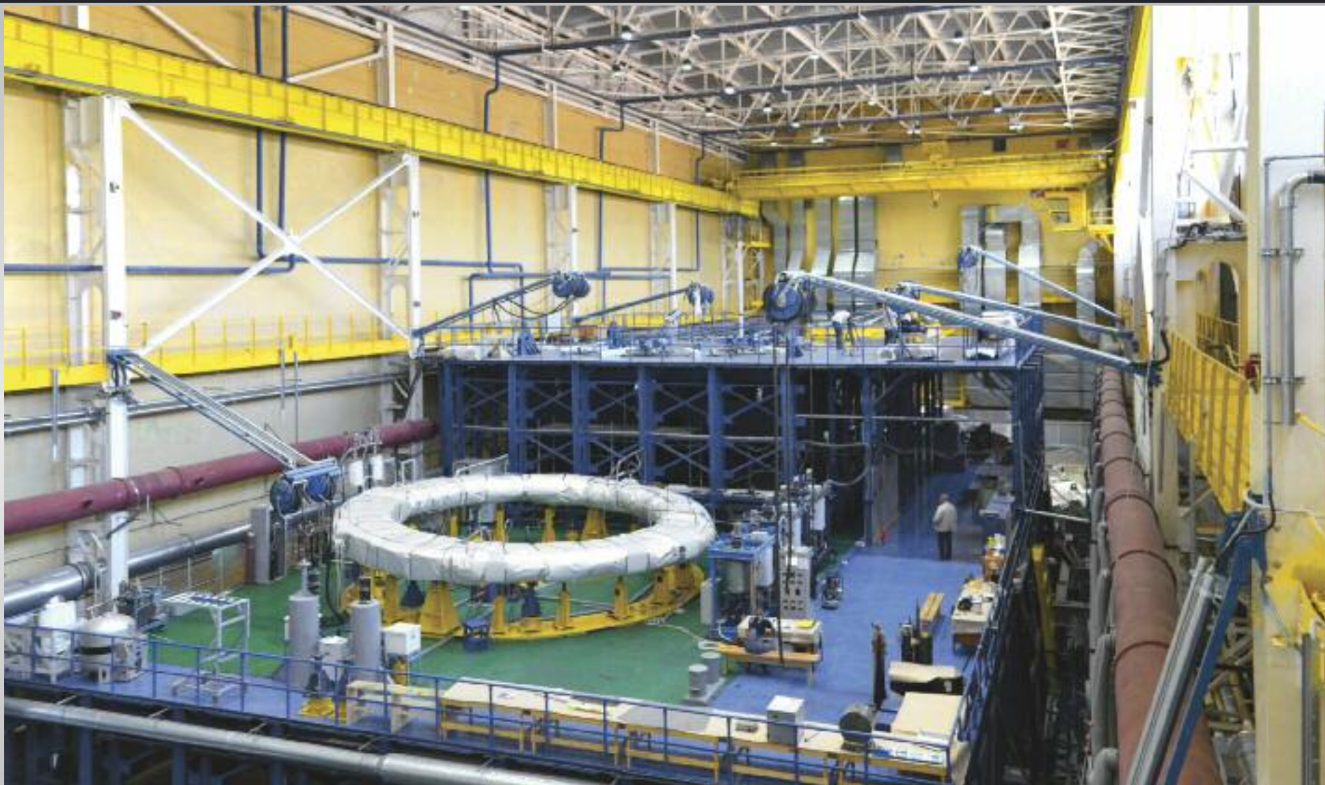
In St. Petersburg, specialists of the Efremov Institute and the Srednensky shipyard have completed the first poloidal field double pancake winding. Eight double pancakes will be stacked to form poloidal field coil 1, the smallest of ITER's ring-shaped magnets.
