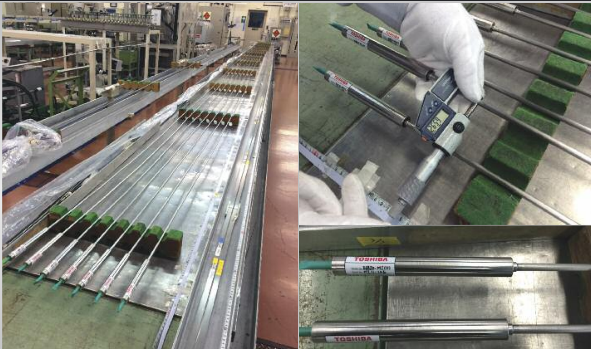
Sealed at both ends, mineral insulated (MI) cables will deliver the signals from the micro fission chambers located near the plasma. The microfission chamber system “counts” the neutrons during operation to measure fusion power.
