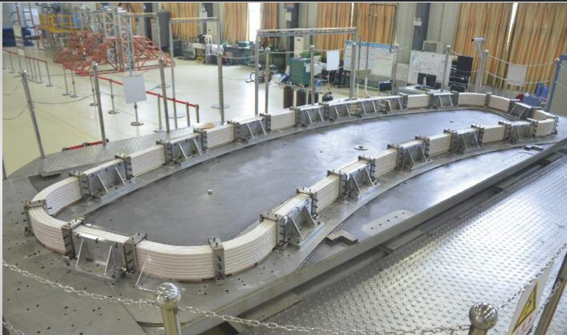
Three sets of six correction coils will be distributed symmetrically around the tokamak to correct field errors. At the Institute of Plasma Physics, Chinese Academy of Sciences (ASIPP), the first-of-series, multiple-pancake bottom correction coil winding is prepped for the wrapping of ground insulation.
