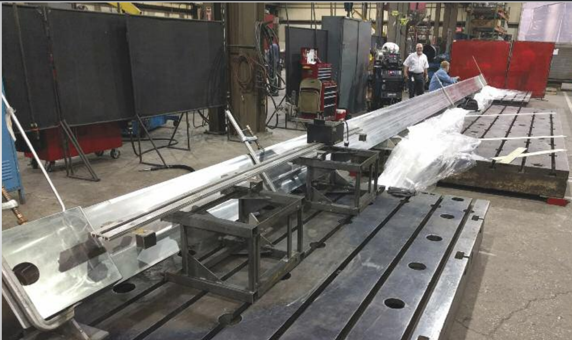
Tie plates for the central solenoid undergo machining at Major Tool and Machine in Indianapolis, Indiana. These plates are part of a specially designed support structure that will hold the central electromagnet in place during operation despite thousands of tonnes of force.
