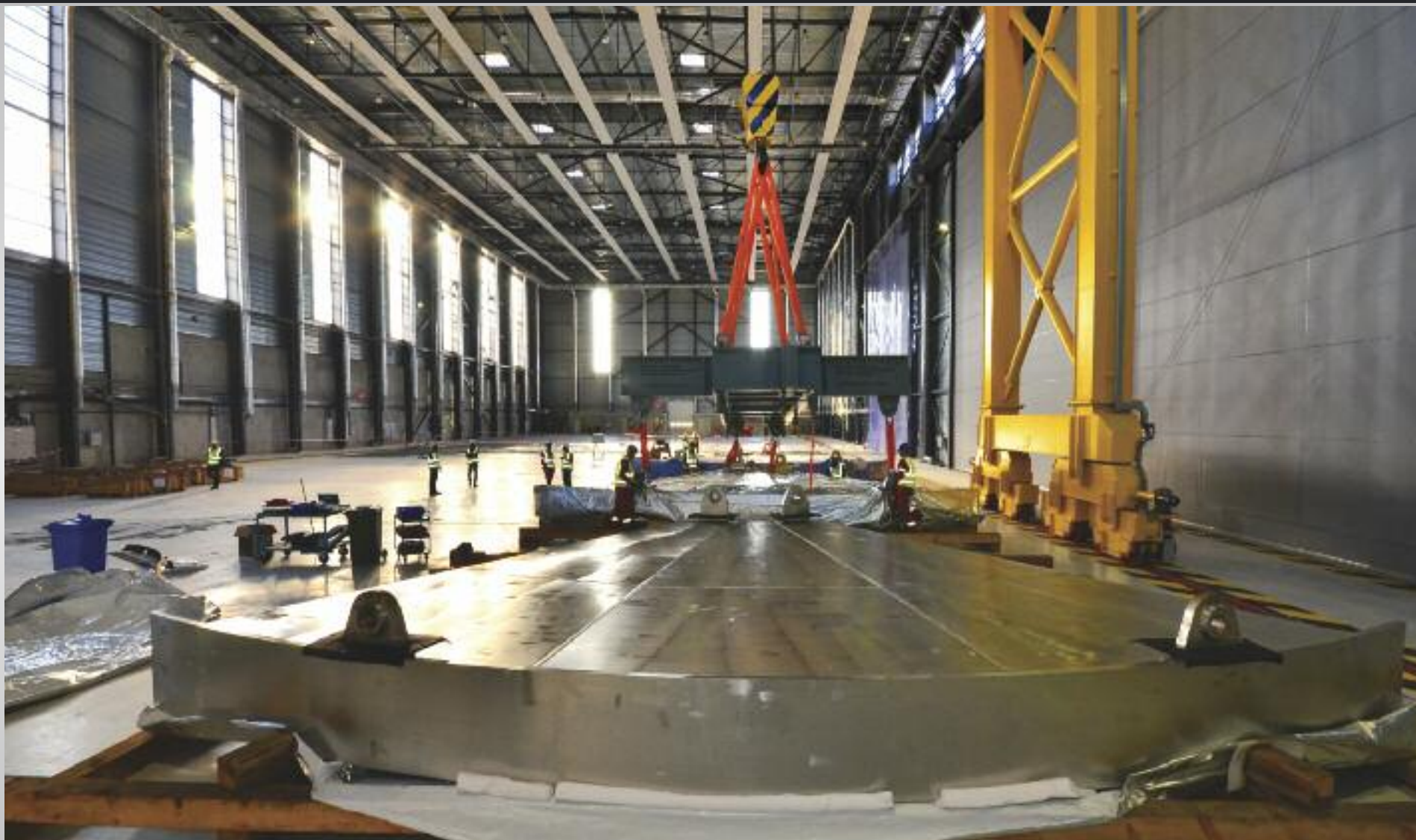
Advanced welding techniques such as automated, all-position narrow groove gas tungsten arc welding have been specially developed for the challenging assembly of 54 segments into the single largest component of the ITER machine. Pictured: two triangular segments for the cryostat base (tier 1) are stored in the Cryostat Workshop. December 2015
