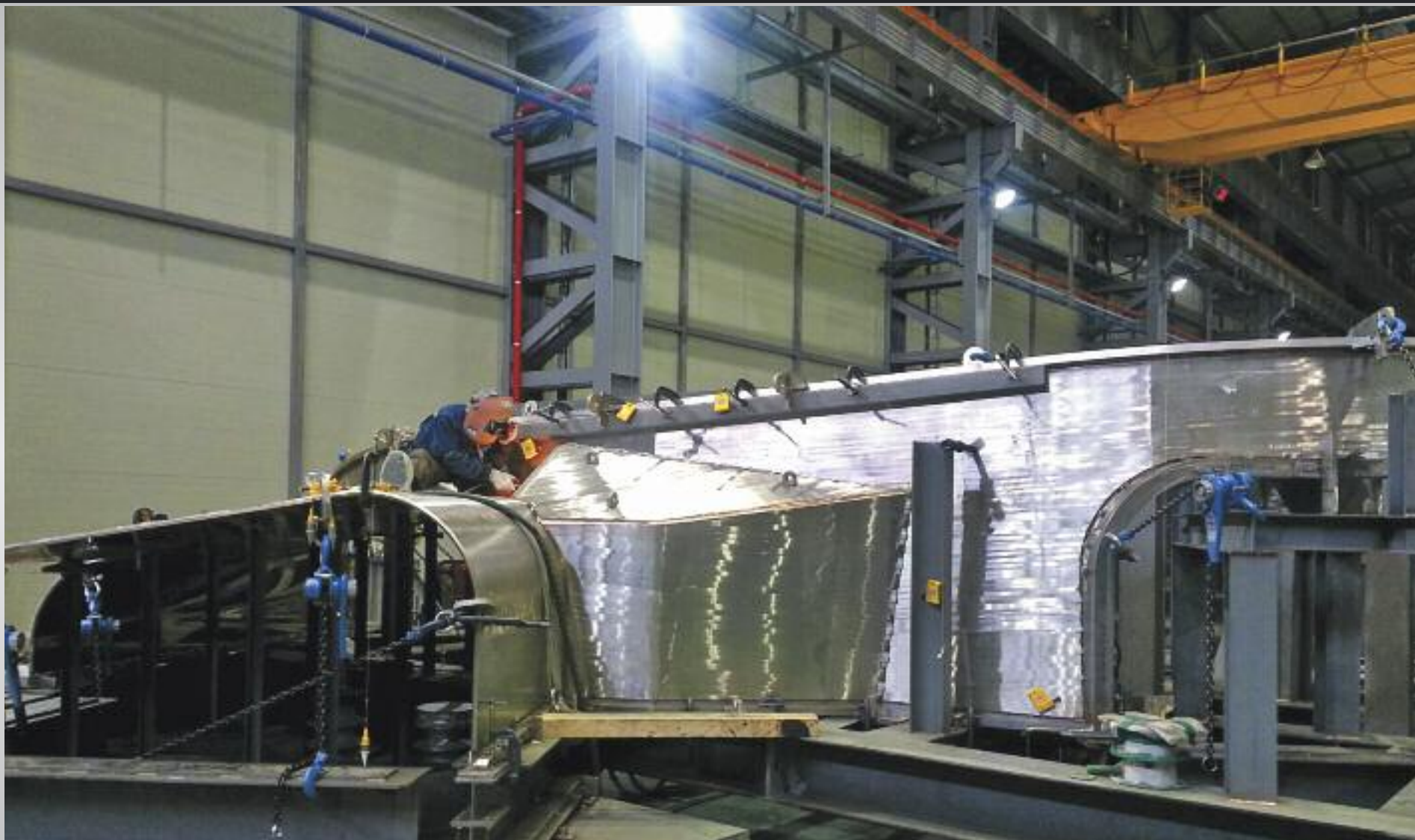
A thin barrier of stainless steel (10–20 mm), actively cooled and covered with a low-emissivity coating of silver, will protect the magnet coils from thermal radiation. At SFA Engineering in Changwon, welding is underway on an outboard sector of the vacuum vessel thermal shield.
