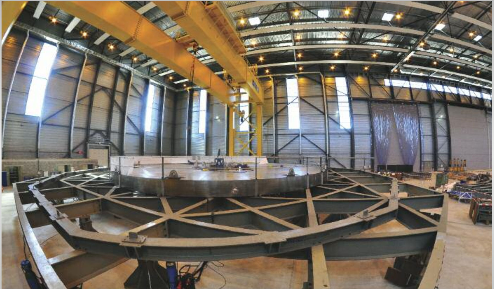
Welding begins on tier 1 of the cryostat base. When assembled with second tier segments, the cryostat base will weigh 1,250 tonnes. September 2016
