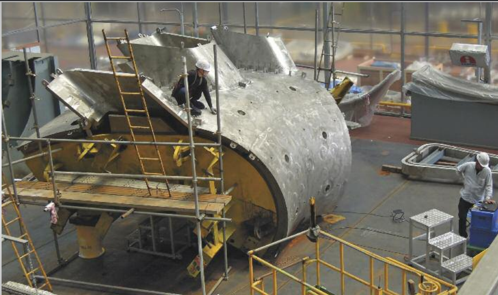
Each of the nine vacuum vessel sectors will be assembled from four segments (upper, lower, inner and outer). At Hyundai Heavy Industries, technicians carry out 3D dimensional inspection on the upper segment of sector 6.
