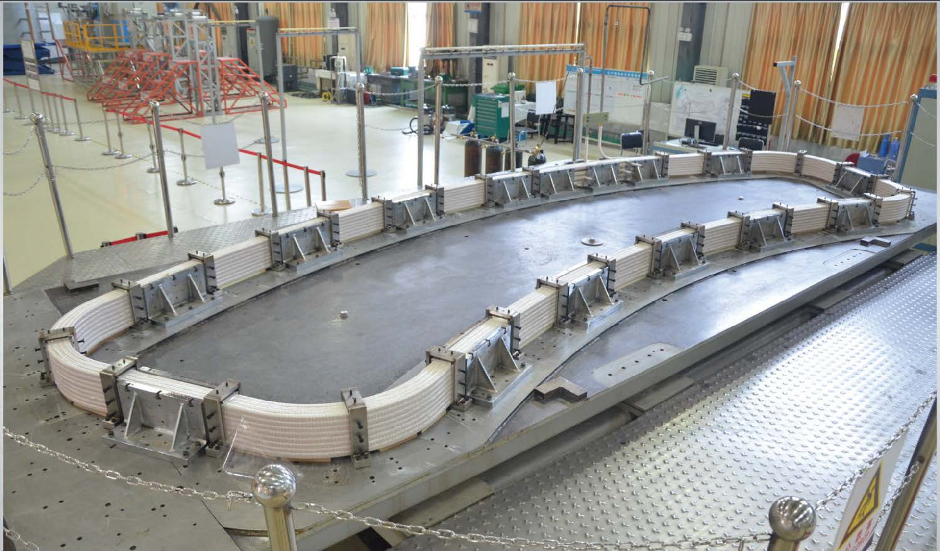
Three sets of six correction coils will be distributed symmetrically around the tokamak to correct field errors. At the Institute of Plasma Physics, Chinese Academy of Sciences (ASIPP), the first-of-series, multiple-pancake bottom correction coil winding is prepped for the wrapping of ground insulation.
