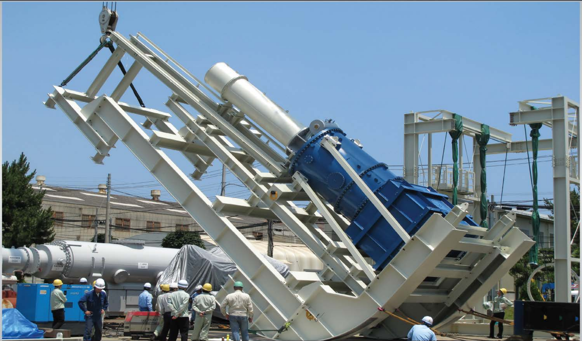
Japan is supplying the high voltage power supplies and the high voltage bushing for MITICA, a full-scale ITER neutral beam injector under installation at the PRIMA neutral beam test facility in Italy. Pictured are assembly tests on the 1 MV bushing at Hitachi, before the component is shipped and installed in the 1 MV insulating transformer.
