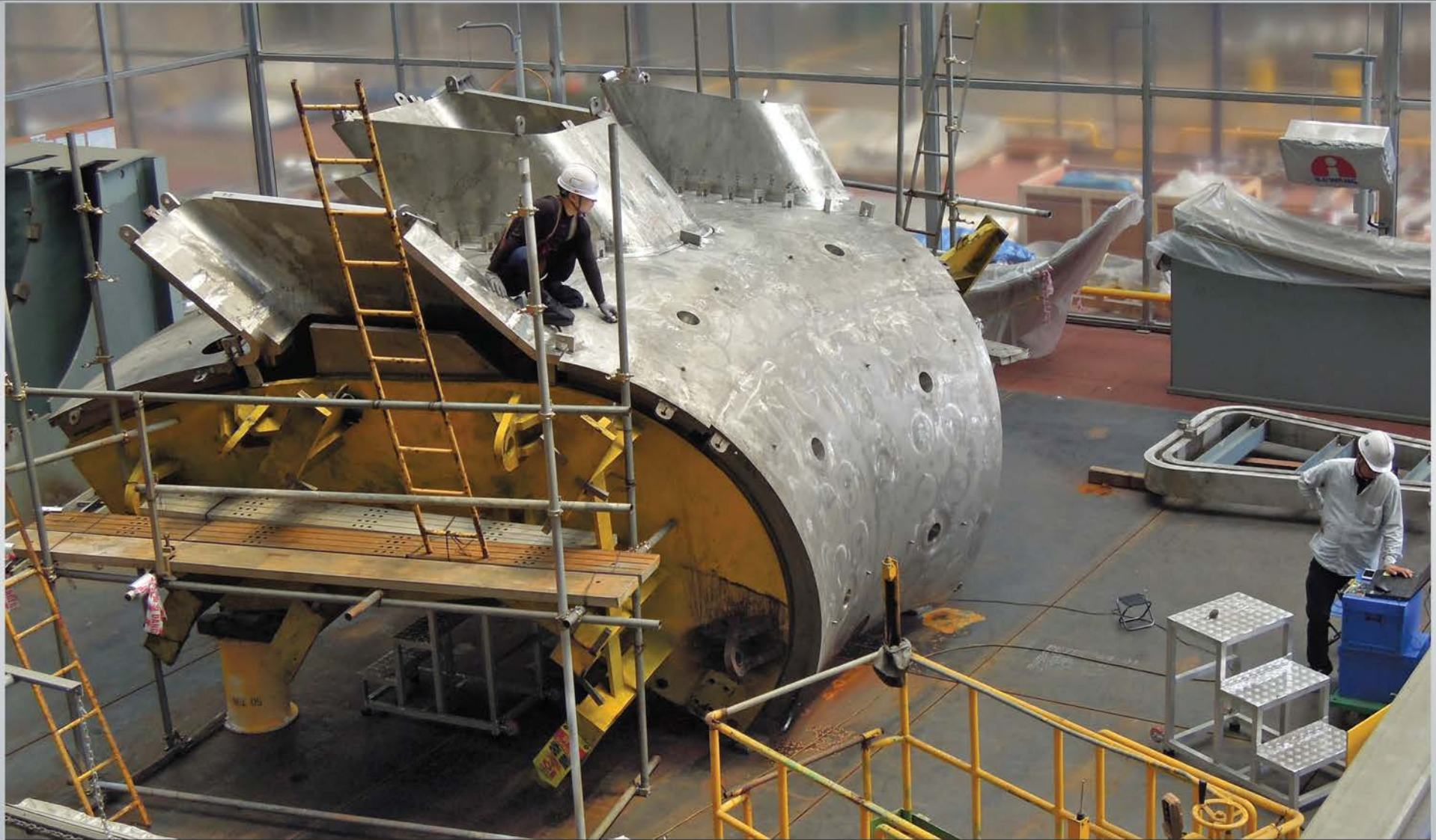
Each of the nine vacuum vessel sectors will be assembled from four segments (upper, lower, inner and outer). At Hyundai Heavy Industries, technicians carry out 3D dimensional inspection on the upper segment of sector 6.
