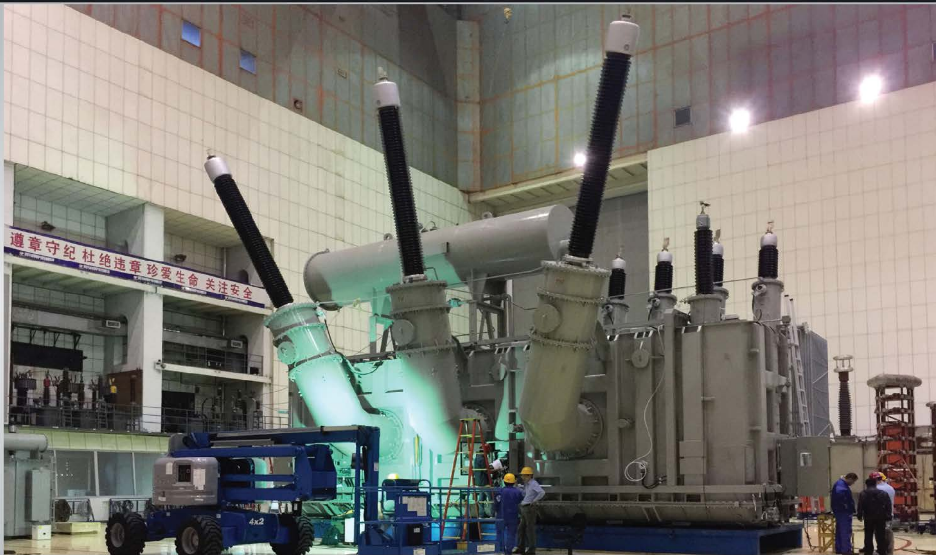
This 300 MVA step-down transformer is one of three that have successfully passed factory acceptance tests in China for ITER's pulsed power electrical network. The first transformer reached ITER in 2016; two others are expected next year.
