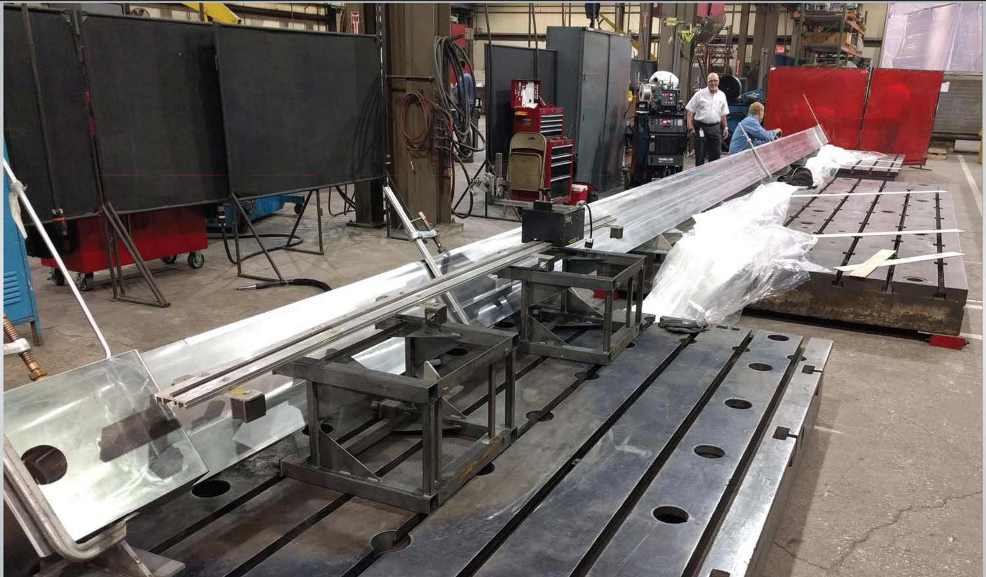
Tie plates for the central solenoid undergo machining at Major Tool and Machine in Indianapolis, Indiana. These plates are part of a specially designed support structure that will hold the central electromagnet in place during operation despite thousands of tonnes of force.
